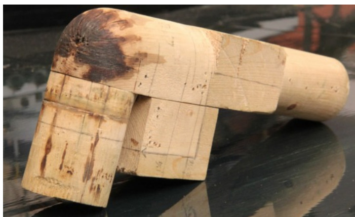
These two photos show how Charles formed the streamlined shroud on his latest locomotives. This form has been used to make 10 locomotive models. You can see how the brass is cut in the right photo. The brass is then formed around the wood and held with copper wire or tape. The joints are then soldered. Then the piece is removed from the form. Charles solders some small pieces to the back side for added strength.
