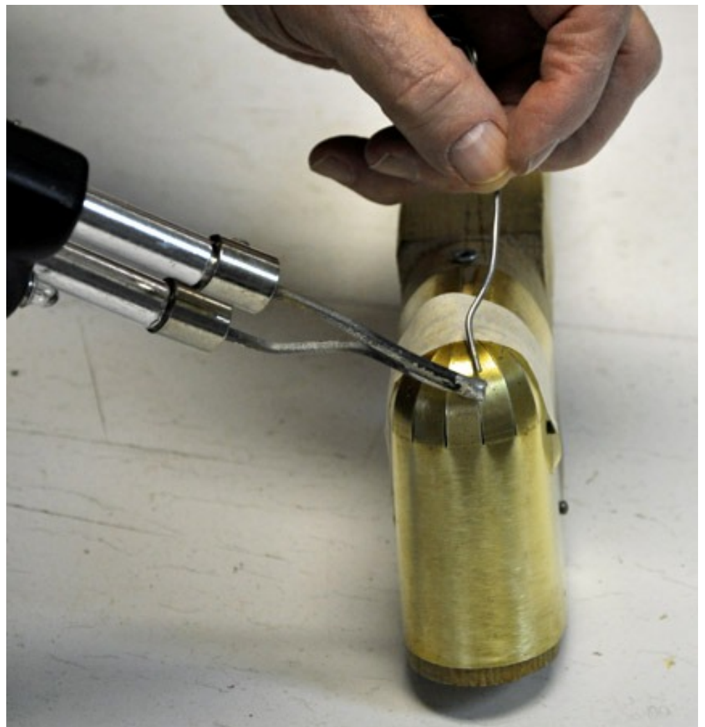
These photos show how the nose of the streamline shrouding on the locomotive was formed. After the brass was formed around the wood form, Charles taped it in place and started soldering the seams.
