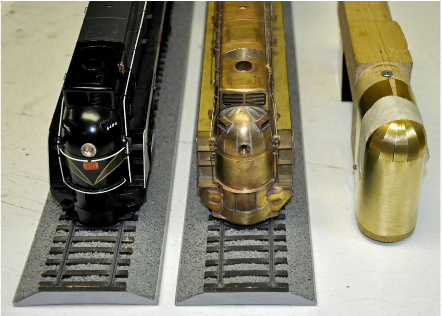
These photos show the progression of the streamline shroud. On the right is the brass on the wood form. In the center is the finished un painted model. On the left is a finished painted model.
