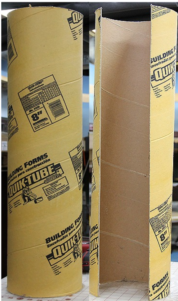
8 inch concrete tube cut to length, and then sliced for the roadbed.
