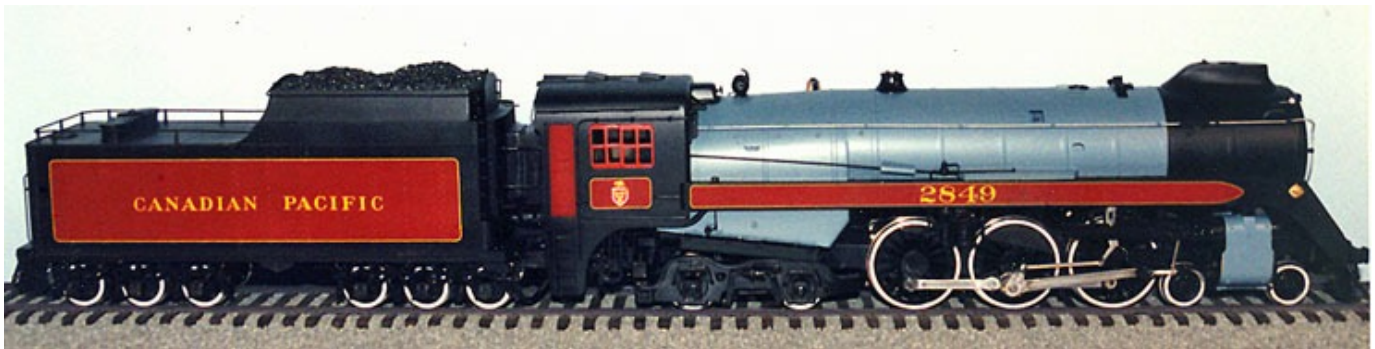
This model of a Canadian Pacific Royal Hudson class H1e hudson type 4-6-4 was the second time Charles built one of these. This model was made in 1998. The prototypes were made in 1937.
