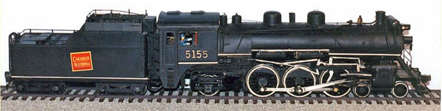
This model of a Canadian National class J4f pacific type 4-6-2 was built by Charles in 1976. The prototypes were built in 1920.
