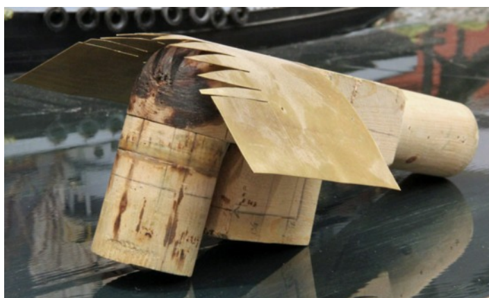
These two photos show how Charles formed the streamlined shroud on his latest locomotives. This form has been used to make 10 locomotive models. You can see how the brass is cut in the right photo. The brass is then formed around the wood and held with copper wire or tape. The joints are then soldered. Then the piece is removed from the form. Charles solders some small pieces to the back side for added strength.
