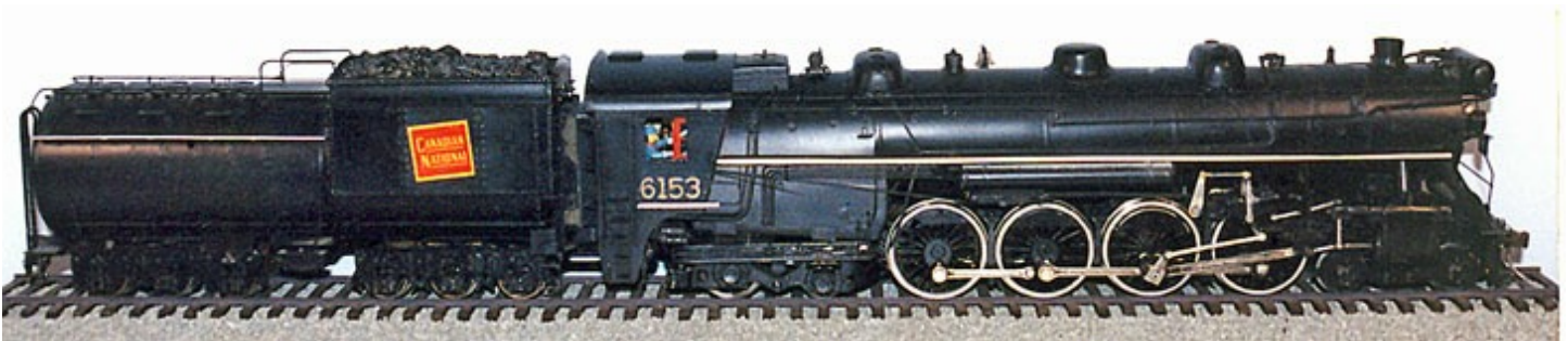
This Model of a Canadian National class U2c northern type 4-8-4 was built by Charles in 1978. The prototypes were built in 1926.
