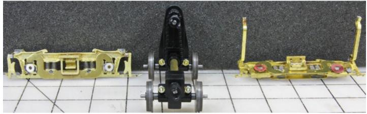
Now we have the truck assembly apart. Note that one sideframe has plastic inserts for the axles, while the other has fiber washers.
