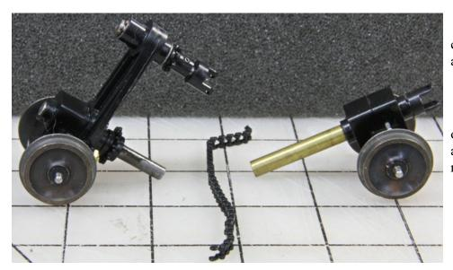
With the sideframes off, you can simply pull the two wheel assemblies apart.
