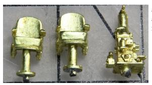
What I was able to do was remove the fan itself for better access to the inside and making it easier to paint. The yellow arrows show where it was soldered on, and it was very easy to remove.
