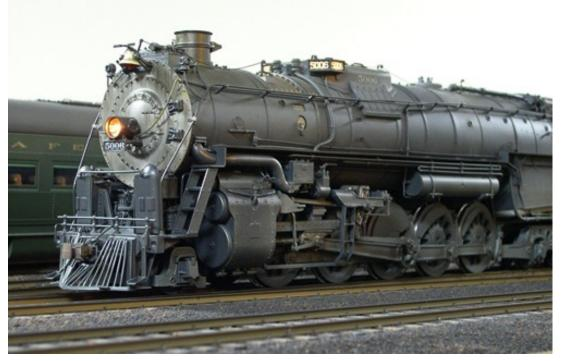
No one has ever imported a Santa Fe 5001 class model in O scale. This is what one might term a "hyperdetailed" model of ATSF 5006. It started life as a USH ATSF 2-10-4. All the detailing was changed along with the wheels and drive train. If something appeared on the real 5006, it is on this model.
