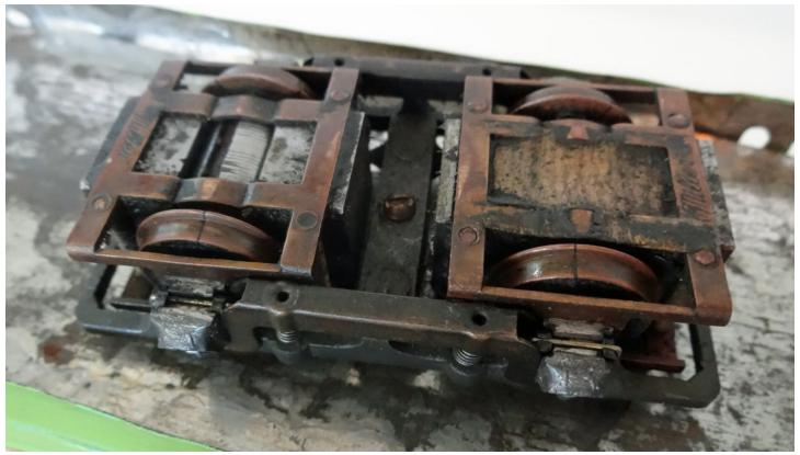
This is the power truck from the PCC model on the previous page. These were made by the Robert L. Miller Labritory in Valparaiso, Indiana for S Scale models. In the early 1950's, they were used by traction modelers in O Scale because they were the only under floor power trucks available. Note that the wheel treads are the armature commutator bars. See the breaks in the wheel tread. One motor is covered with masking tape. Photo by Ed Halstead.
