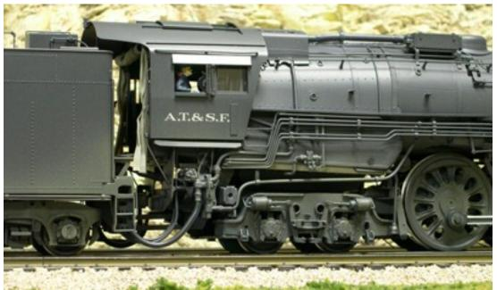
This is a Sofue ATSF 3460 class Hudson *super-detailed to exactly* match ATSF 3461 around 1950. The original model was exquisite, but some things could be upgraded including the engine to tender connections you see here. New castings from PSC and some piping changes were done before painting, lettering, and weathering.
