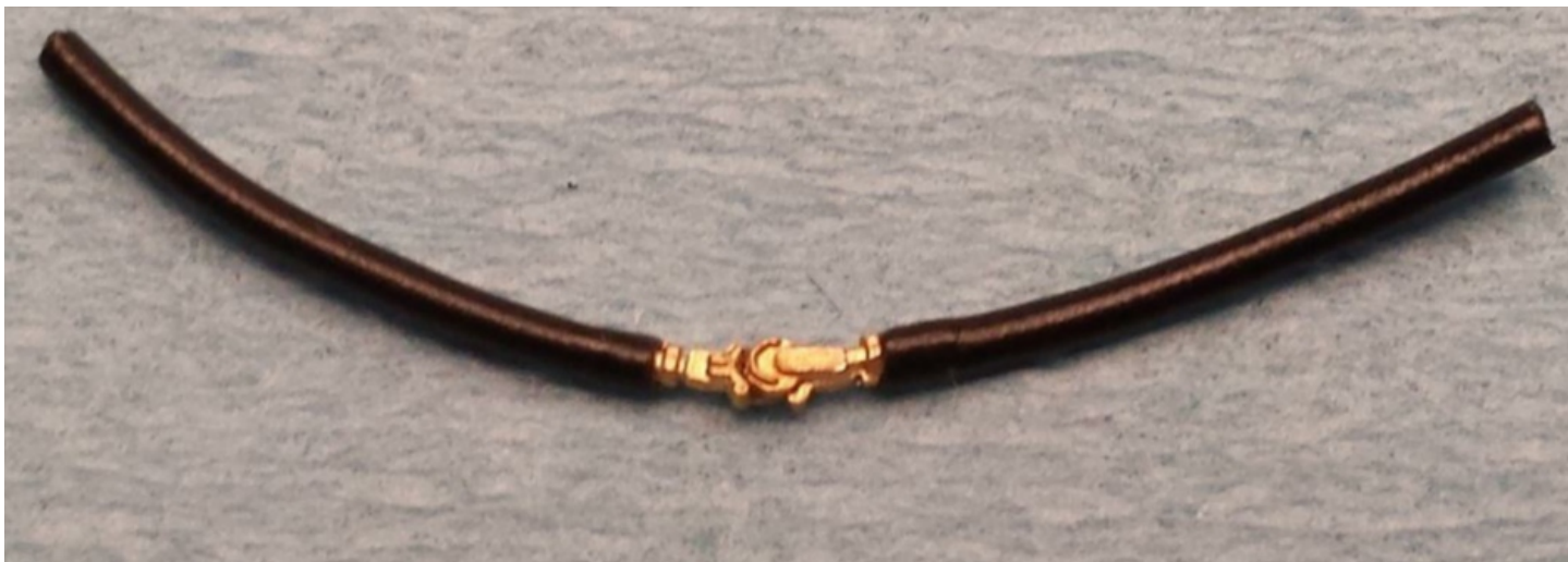
Figure 5 These are the finished MU Hoses that Bob uses. The glad hands are glued, and this whole unit is removed from the model when the units are changed.
