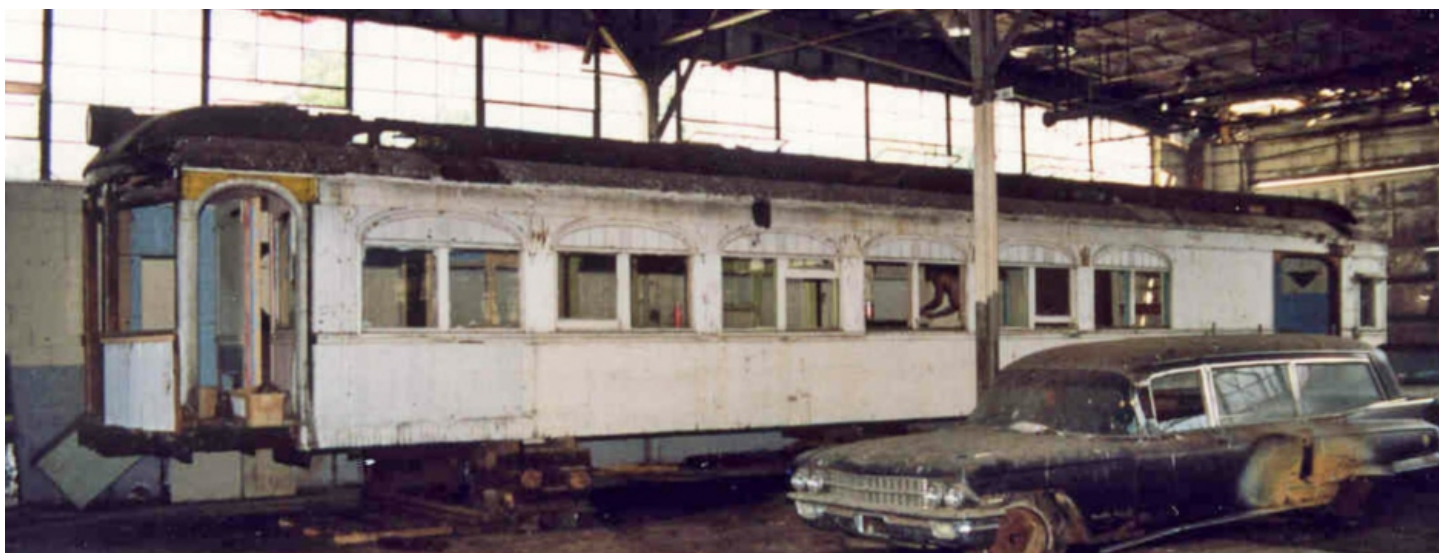
This is how the car looked when I first saw it to do the survey. At first glance it looks grim, but there is actually a lot here. The car was still straight and that's good. Since the car is made of wood, it is easy to repair or replace parts. There is also enough of the car that dimensions can be obtained and parts replicated. Most of the framing in the car today is original. What we had to replace was everything on the exterior. The interior woodwork is still there, but we did need to make new partitions to replace the ones that the homeowners and railroad had removed.
