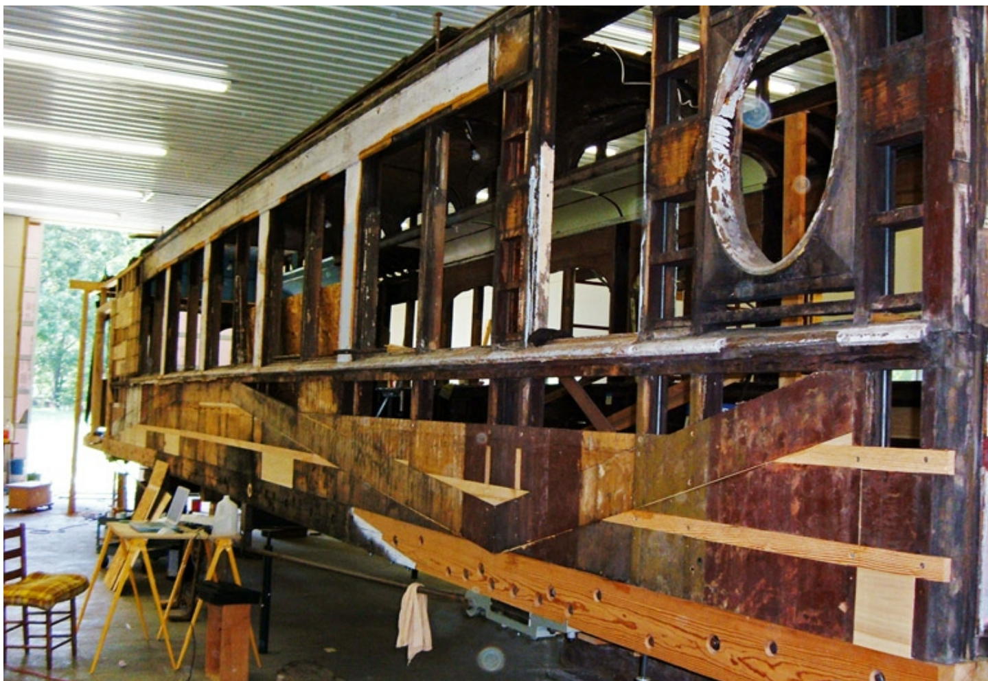
Here is the left side of the car as we were working on it. You can see the wood truss built into the side of the car. This truss was mostly for sway bracing. The truss rods do most of the work supporting the car.
