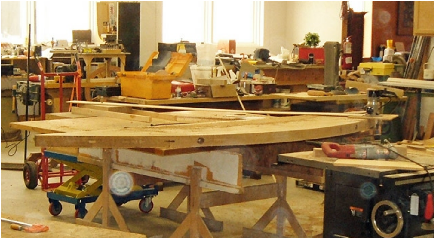
This is the set up I made to cut the large radius of the rear end beam of the car. These pieces are made of 3 inch thick white oak that is splined together for alignment and then through bolted with threaded rods. The router is mounted on a long stick that pivots at the center of the circle. You have to make a lot of little cuts but it works.
