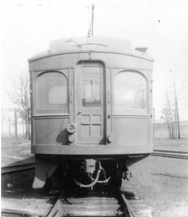
These two photos are probably also valuation photos. Note the pilot on the front end view on the right. The wood pilot has been replaced by a steel wedge pilot.
