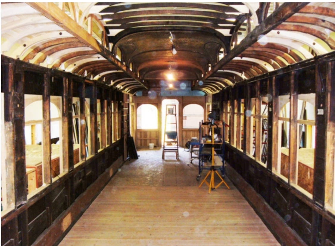
Here is the left side of the car as we were working on it. You can see the wood truss built into the side of the car. This truss was mostly for sway bracing. The truss rods do most of the work supporting the car.
