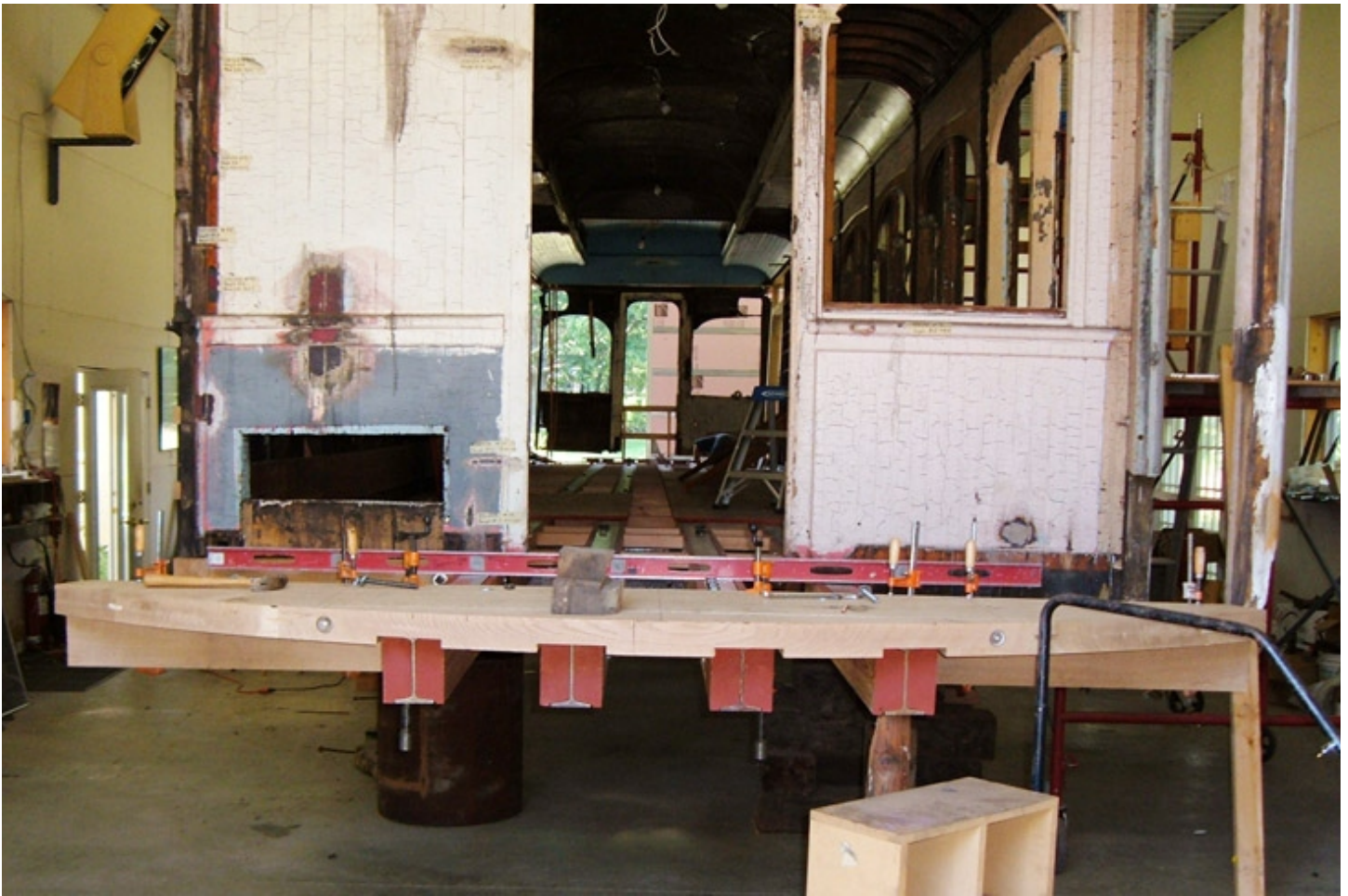
Here is the rear end beam in place. Note how the steel “I” beam sills have wood wrapped around them. This was common in electric railway construction. The reason for the wood is to provide a mortise to locate the frame spreaders and a place to nail the floor to.
