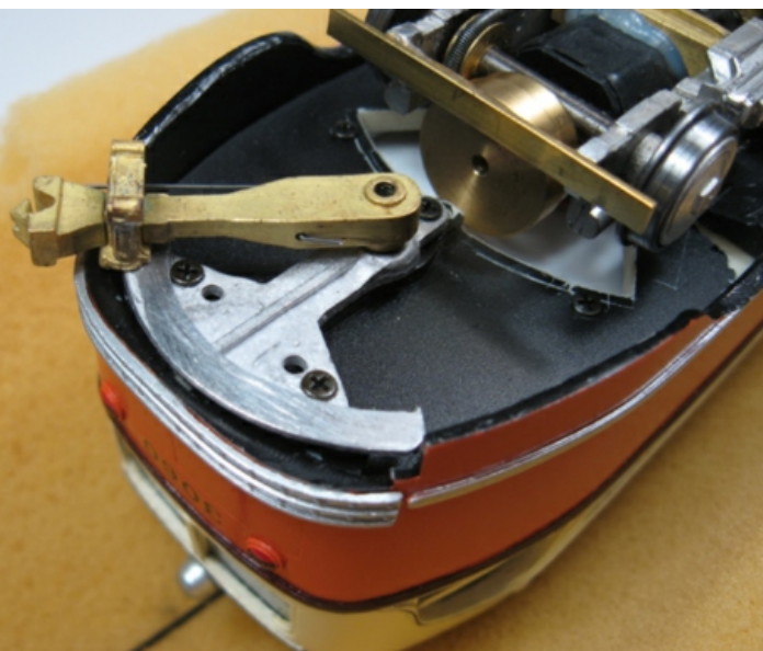
Photo 11 showing the rear radius bar and coupler mounting.
