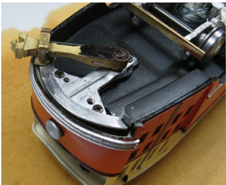
Photo 10 showing the new front radius bar and coupler mounting.
