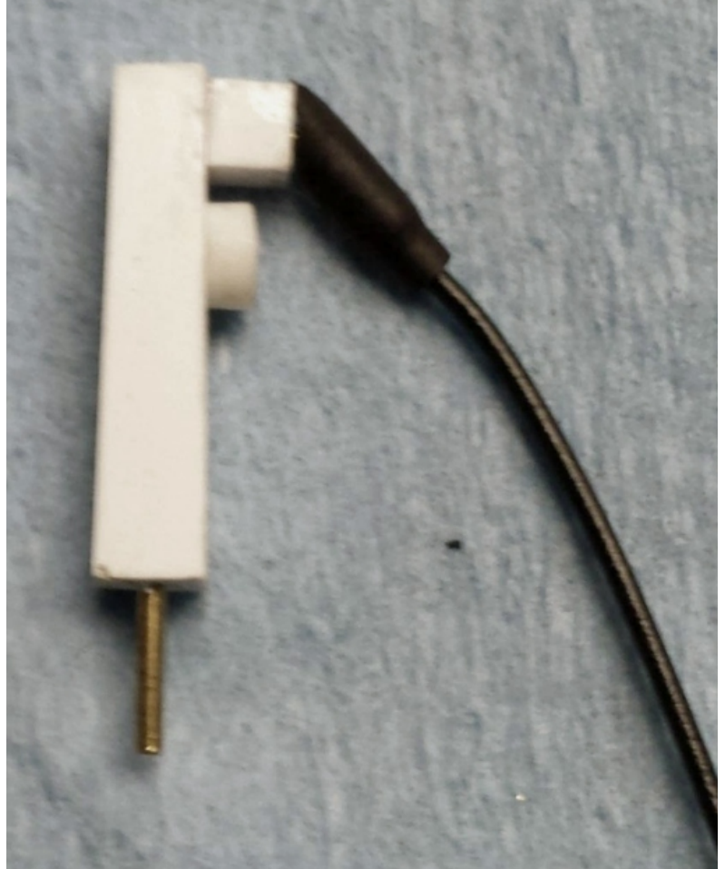
Figure 4 This is how the finished MU stand looks. The black "cable" can be removed when the units are uncoupled. The white styrene stand now gets glued to the pilot of the locomotive.
