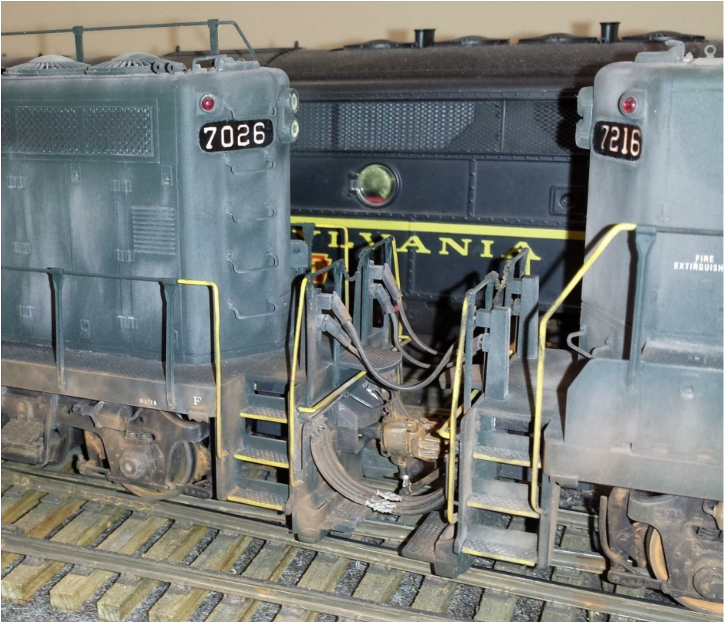
Figure 1 This detail photo of two contest winning Red Caboose GP-9 models that Bob built shows the multiple unit connections that are installed.
