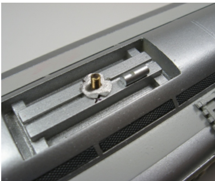
Photo 12 showing the mounting stud for the working trolley pole on Charlie's model.
