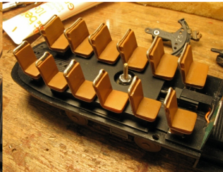
Photo 7 When the motor cover was painted and installed, Charlie trimmed the legs on the seats and installed them. The seats are visible on the finished car and you cannot see the motor cover.
