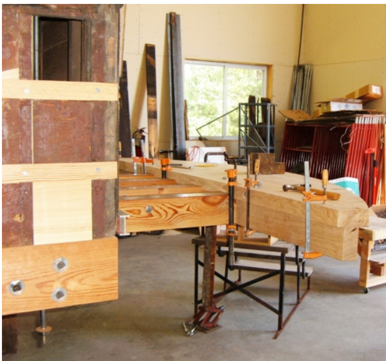
The end beam sits on the center and intermediate sills and is notched where the sills are. Here, Gary is cutting the notches with the router. When these cars were made, the shops had large gaining saws for doing this work. We had to bring the tools to the work.
