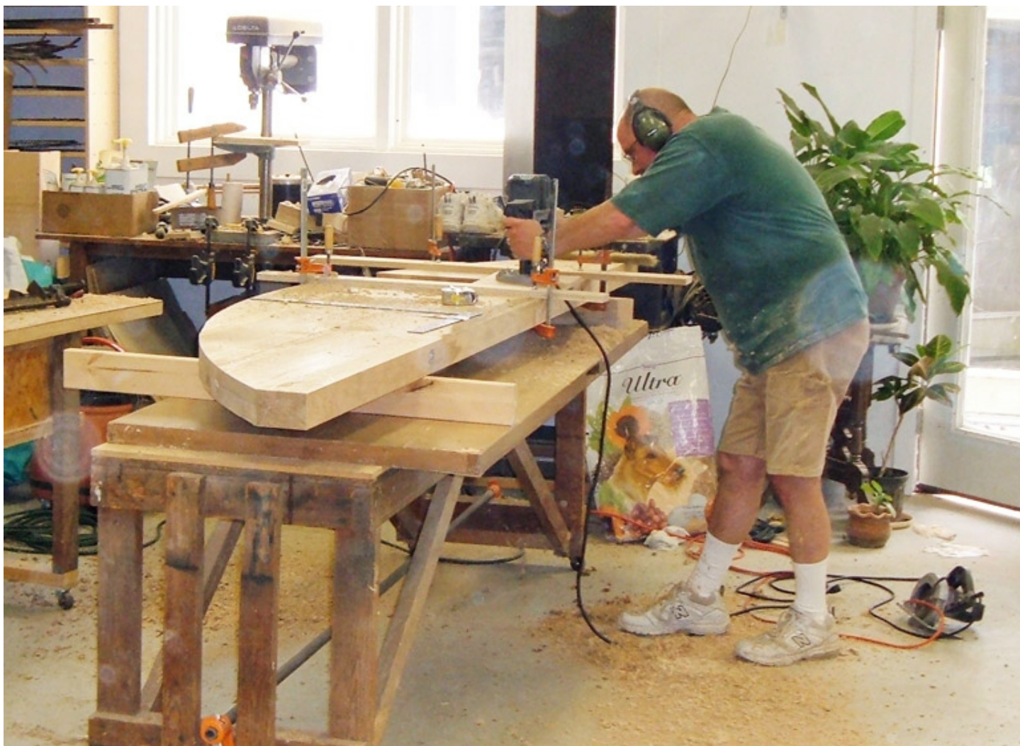
The end beam sits on the center and intermediate sills and is notched where the sills are. Here, Gary is cutting the notches with the router. When these cars were made, the shops had large gaining saws for doing this work. We had to bring the tools to the work.
