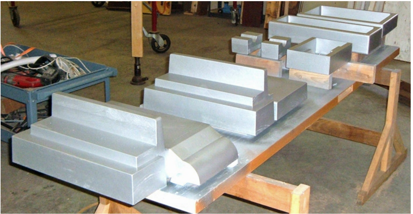
These are the parts of the pattern after I sealed them. They are now ready to go the foundry.
