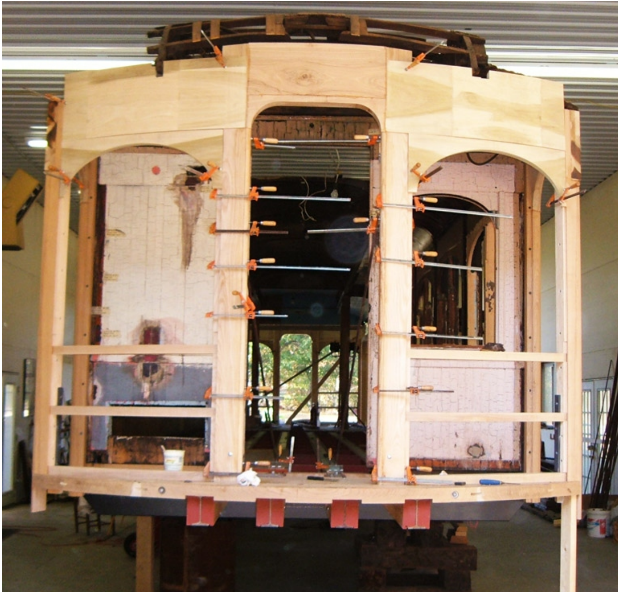
Here we are finishing out the rest of the framing at the rear of the car.
