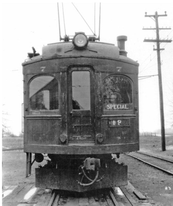
These two photos are probably also valuation photos. Note the pilot on the front end view on the right. The wood pilot has been replaced by a steel wedge pilot.
