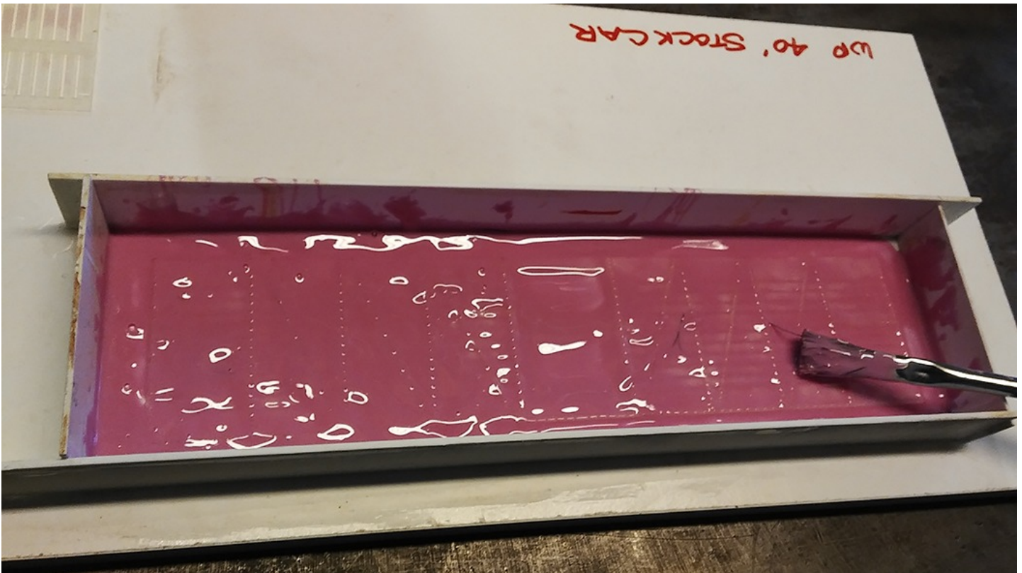
Silicon rubber is brushed over the side pattern. This process takes time and patience to avoid any bubbles or voids up against the part.
