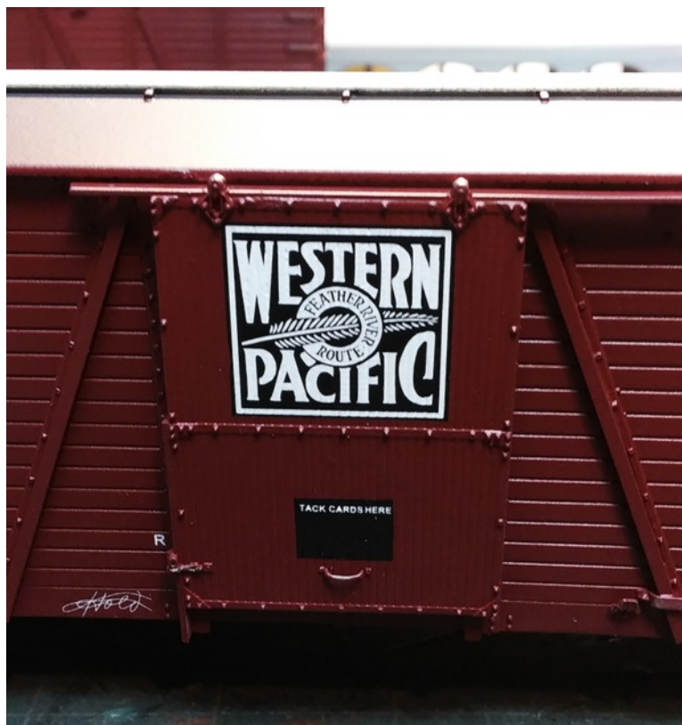
Detail on the door showing the various "fussy" parts, including hangers, latches, and handle. The decals for this car came from a Protocraft set for a later steel car.
