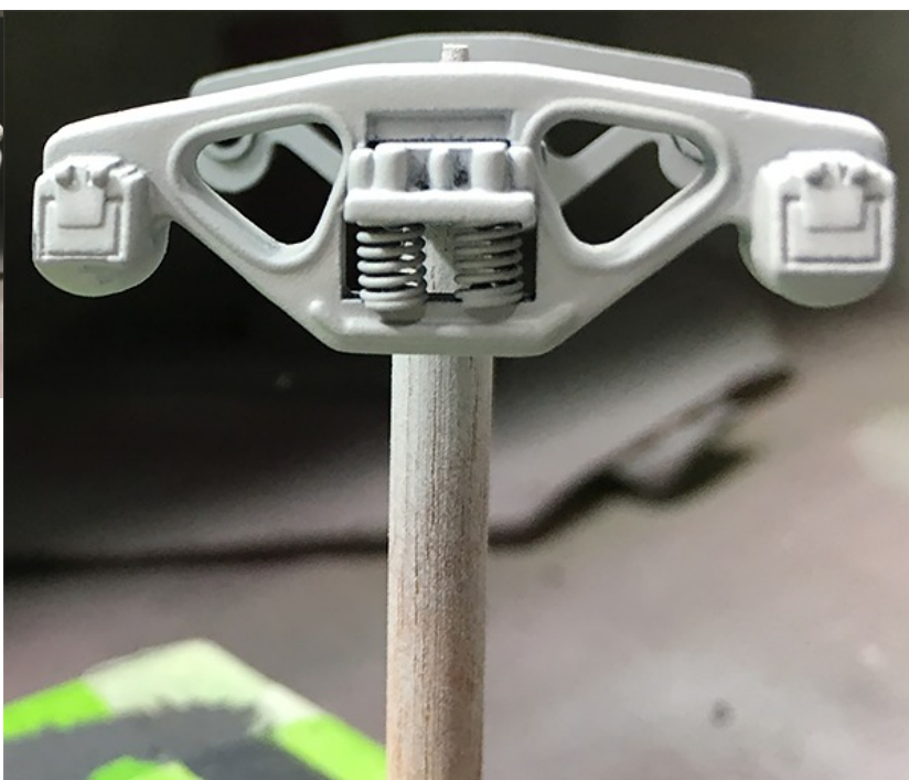
Cutting painters tape about the width of the wheel tread. Once wrapped, they were shot with roof brown.
