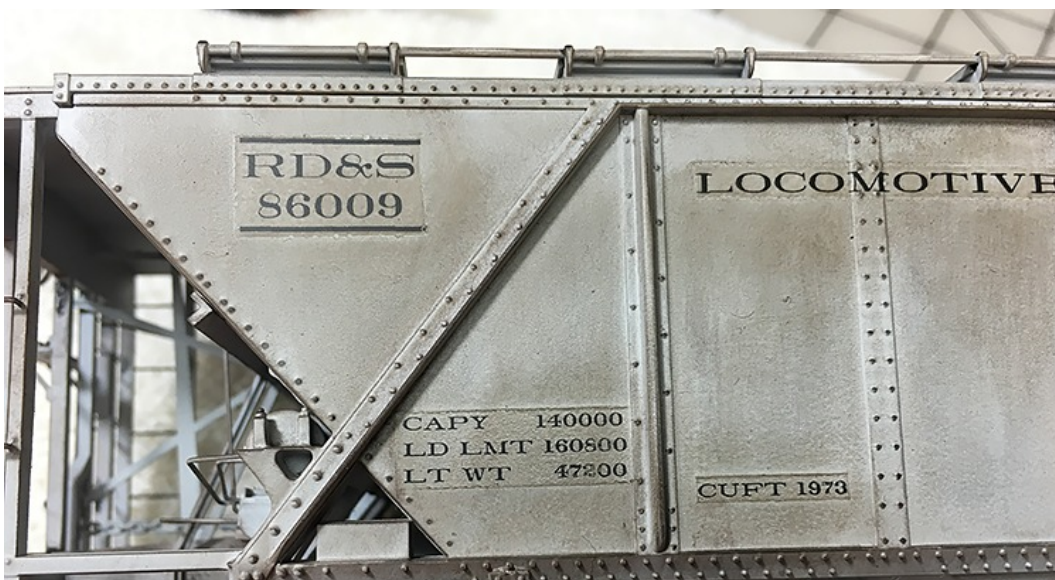
Close up of the problem with the decal film edges and weathering powders.
