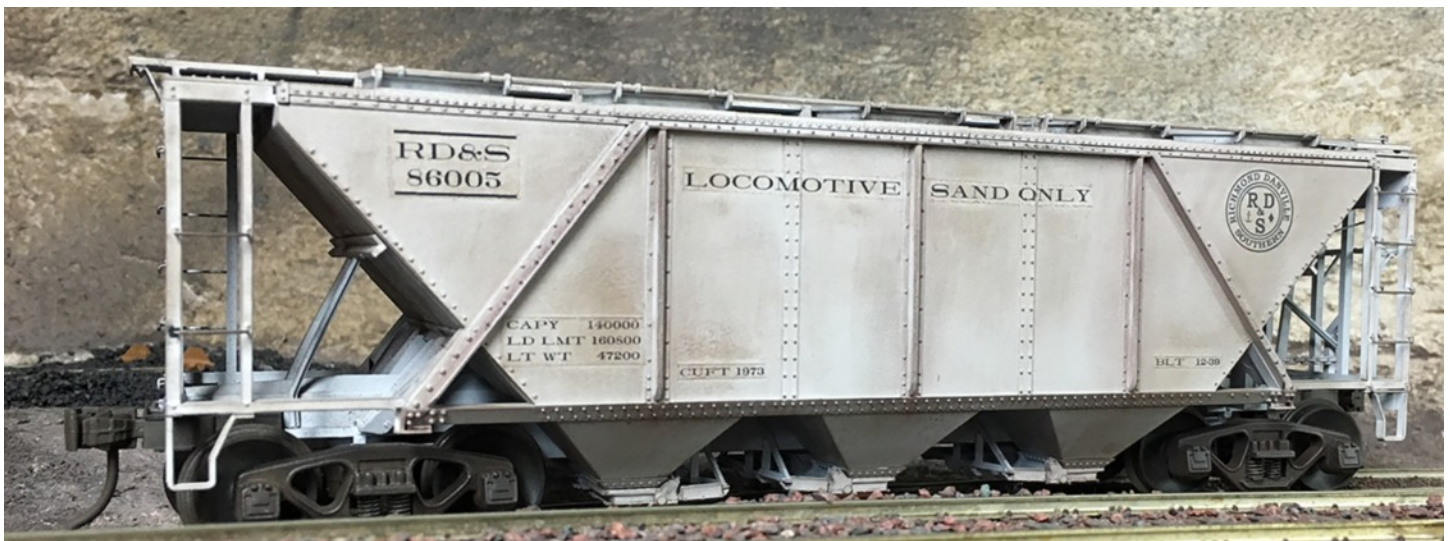
Really ugly decal edges showing up after weathering – all because I did not do what I should have in the beginning.
