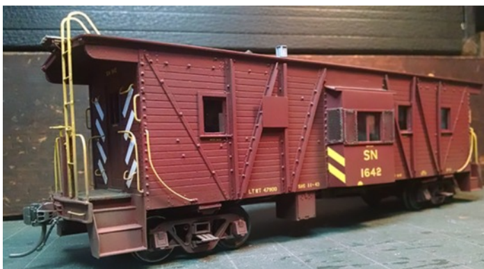
The WP and its subsidiaries, in this case the Sacramento Northern, rebuilt a number of the Pullman boxcars into cabooses. This is an example of one of the bay windows.
