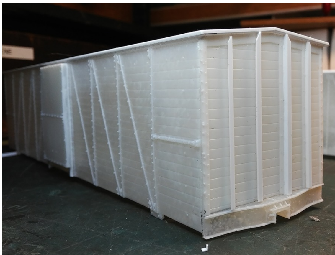
The end of the carbody shows the .062" angle glued in place to create the Zee bracing. Notice that the angle is not in place on the sides. The bolted portion of the Zee brace is cast into the side of the car.
