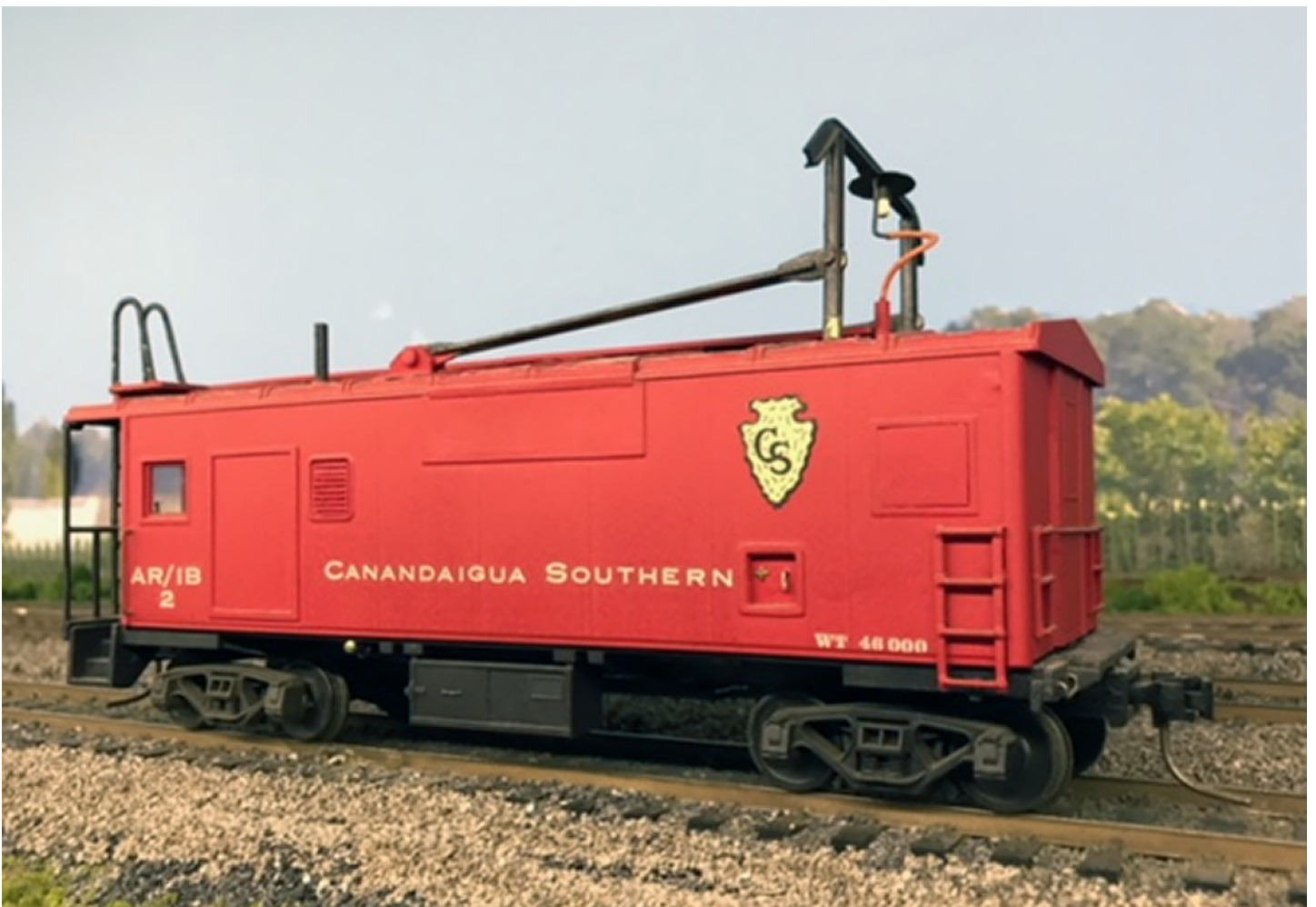
Photo 2: John Armstrong built an icicle car, based on a Southern Railway prototype which mounted a bar at maximum clearance height to knock off icicles in tunnels to prevent damage to automobiles being transported in open auto racks. John kitbashed his model from an Atlas caboose and miscellaneous parts. The bar could be raised and lowered.
