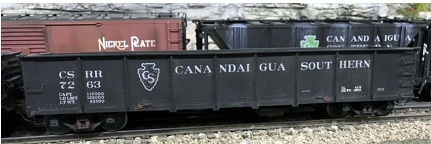
Photo 10 above: CSRR 7263 is a steel USRA design 40' steel gondola. Although still in old lettering, 7263 is a newer design than 7567, shown in another photo. This model was built from a West Shore kit, which may still be available from Funero and Cumerlingo.
