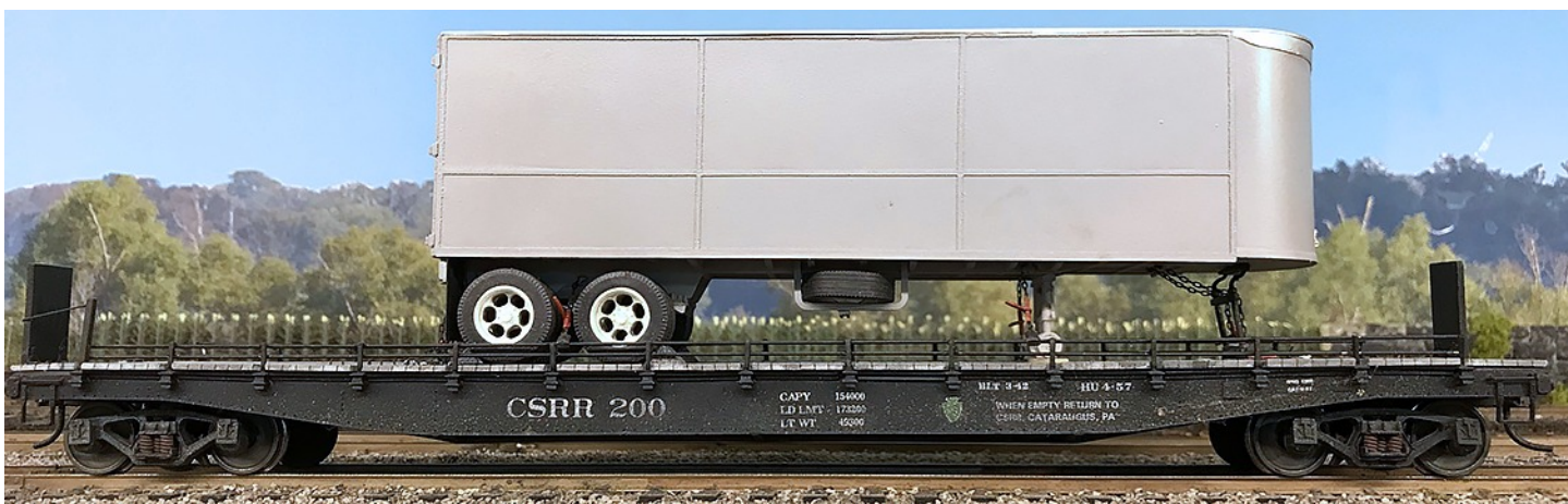
Photo 12 above: CSRR 200 is the class car for 50 52' flat cars converted in 1956 to piggyback service. The car is configured with rub rails and chain tie downs, before king pins were adopted. The car and trailer (not yet lettered) were built from a Berkshire Valley kit originally produced for SONC 1998. Again, these cars are long out of production, but show up regularly at swap meets.
