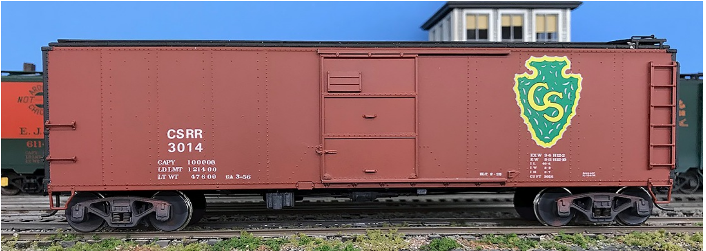
Photo 8A above: CSRR 3014 is an example of one of the comparatively few X-29s rebuilt by the railroad and repainted in the new, sans-serif lettering and billboard herald. Note the overspray on the trucks, a common result of shop rebuilds. When rebuilt, black car cement, and asphalt-like coating, was applied to the ends and roof. This is an Atlas X-29. Custom decals were used for the lettering.
