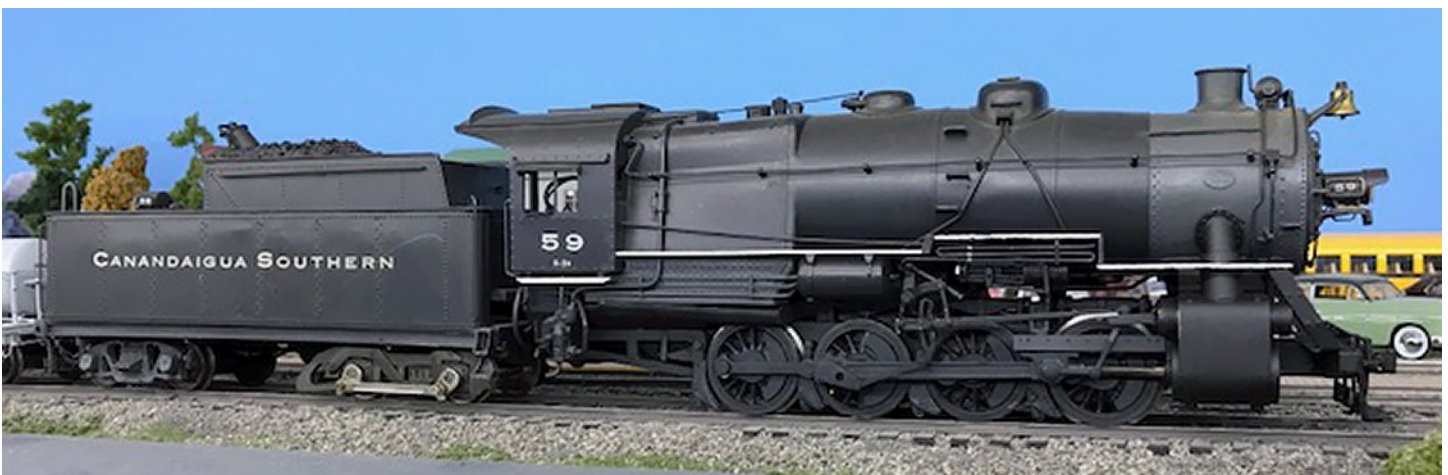
Photo 7B below: CSRR 59 is an 0-8-0 kitbashed by John from USH PRR C-1. It has a different tender, with a booster engine for extra starting power. From a comparison of CSRR 59 and 1206, the family resemblance between CSRR engines can be detected.
