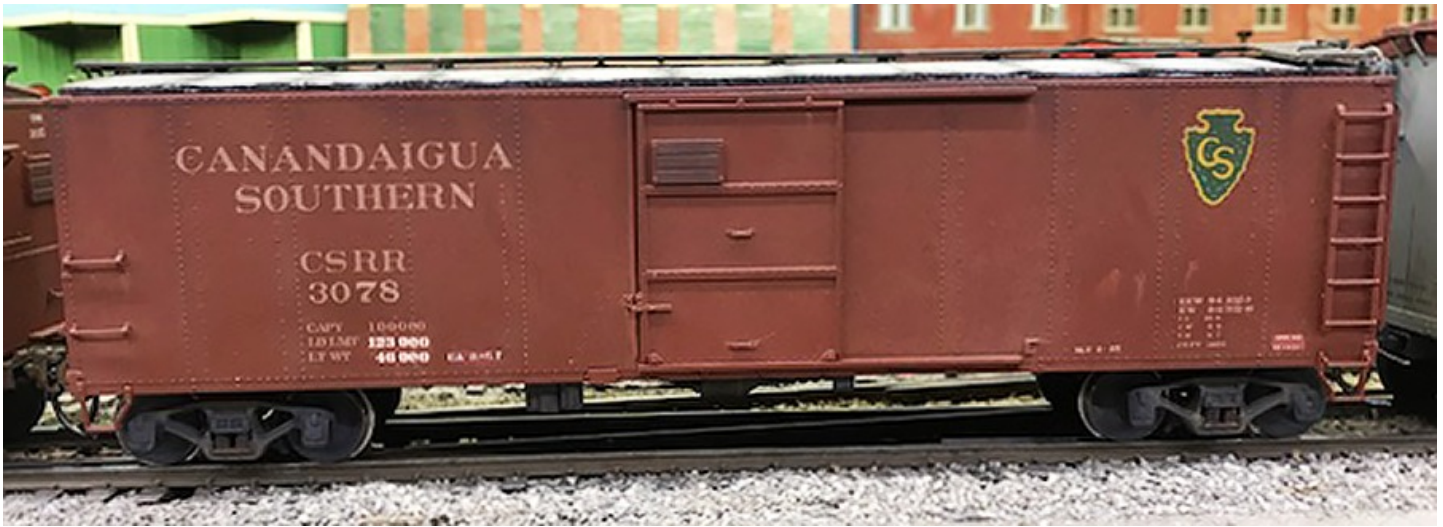
Photo 8C above: CSRR 3078 is an Atlas X-29, custom lettered and weathered. The car is modeled with a galvanized roof, which starts life silver gray, weathers to a dull gray and then develops rust. Roof ribs were non-galvanized steel and might be painted or covered with car cement. It has been reweighed (the newer lettering on the dimensional data) and the journals repacked (the smaller, brighter block on the lower right). The exposure to weather has dulled the white lettering and the outlined herald.
