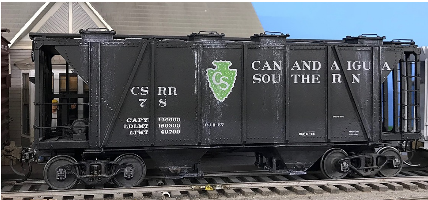
Photo 9 above: CSRR 78 is a covered hopper, built after WWII. As was the case with a number of railroads, CSRR's marketing department was anxious to publicize these new cars and had them numbered beginning with CSRR 1. CSRR borrowed a proven Dispatch Shops design, but utilized 50 ton National Type B trucks, a choice shared by only one other covered hopper order (ATSF). The model is built from a West Shore resin kit, no longer in production, but available from time to time at swap meets and may have possibly been reissued by Funero and Cumerlingo.
