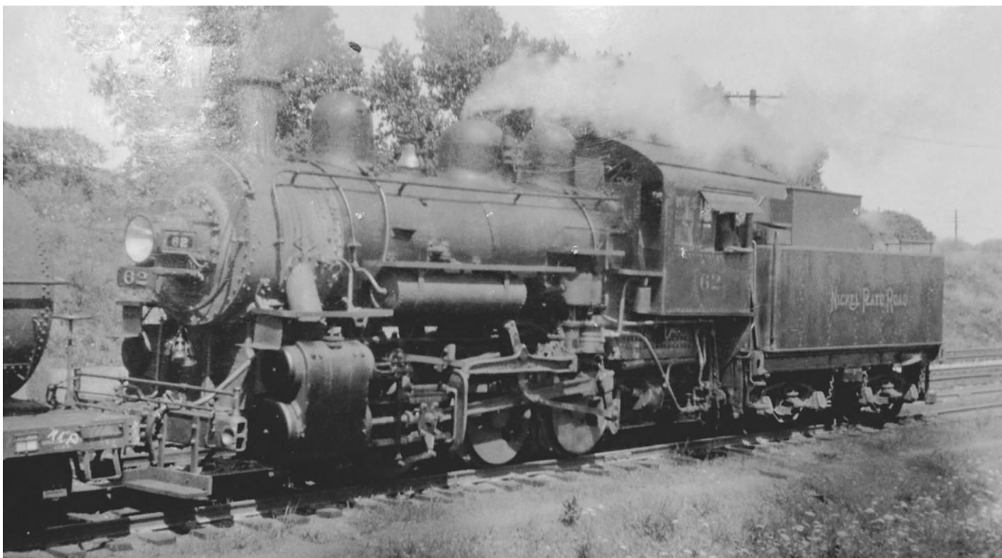
This was the other photo I worked from. The locomotive is a B-11b class of 1917 from Lima and a sister locomotive to the #64. Look close at the details between the two locomotives. They were built at the same time and left the factory the same. They did not stay the same.
