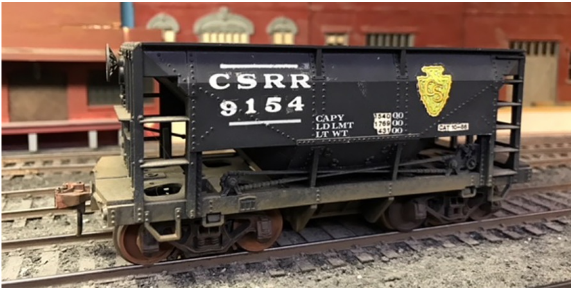
Photo 3 above: CSRR 9154 is an ore car, a stock early 1970s Atlas model with custom decals applied. For reasons unexplained, the herald is yellow and green. The capacity-related stenciling has been painted over, with changes indicated. Such changes can come about when a car is repaired, when trucks or other components are replaced or when journal bearing size is increased or the allowable loading for existing bearings.
