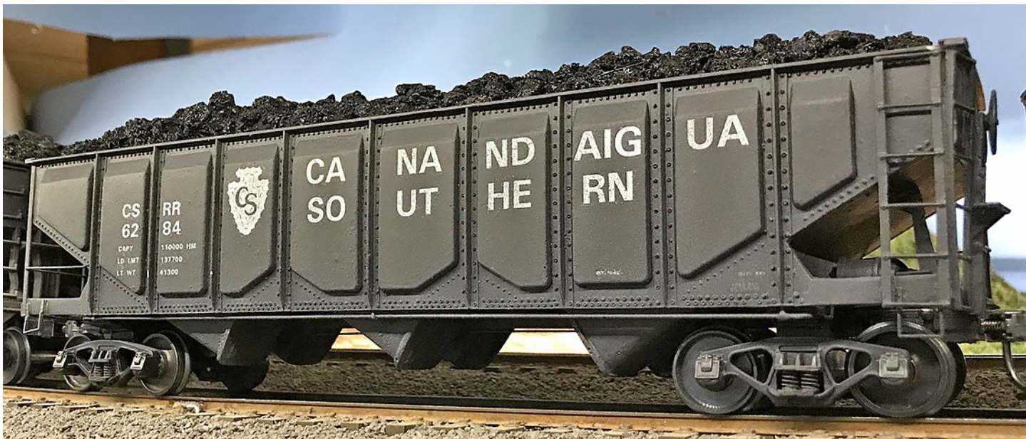
CSRR 6284 is another 70 Ton panel side triple hopper from the 6100-6300 series. This older car has been repainted in the new, sans-serif lettering. It is coupled to an offset-side 70 Ton hopper lettered for Allegheny Midland, Tony Koester's former railroad.
