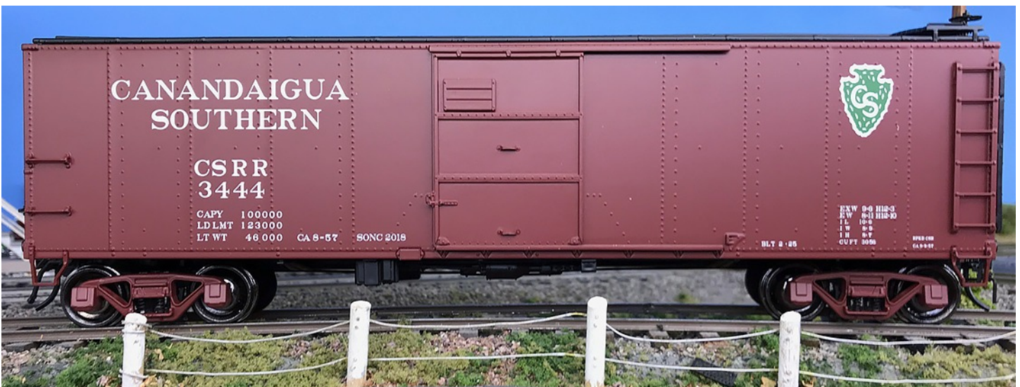
Photo 8B above: CSRR 3444 is an X-29 from the custom run Atlas did for the 2018 Scale O National Convention and presently available through the Website ( http://2018oscalenational.com ). These models are available in three road numbers and in both two-rail and three-rail. CSRR “borrowed” the PRR X-29 construction drawings, but did not use the PRR trucks. Compare 3444 with 3078 elsewhere in the article. The Convention special run is identified by small lettering “SONC 2018” to the left of the door. The roof and ends of the cars are done in black car cement.
