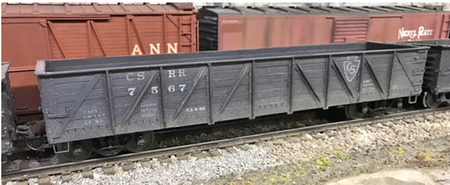
Photo 11 above: CSRR 7567 is a USRA design 40' composite gondola. The car is getting toward the end of its service. Using older prototypes in the same service as newer models gives the impression that the railroad has been operating over an extended period. The model is built from a resin kit offered by Des Plaines Hobbies and represents a PRR prototype.
