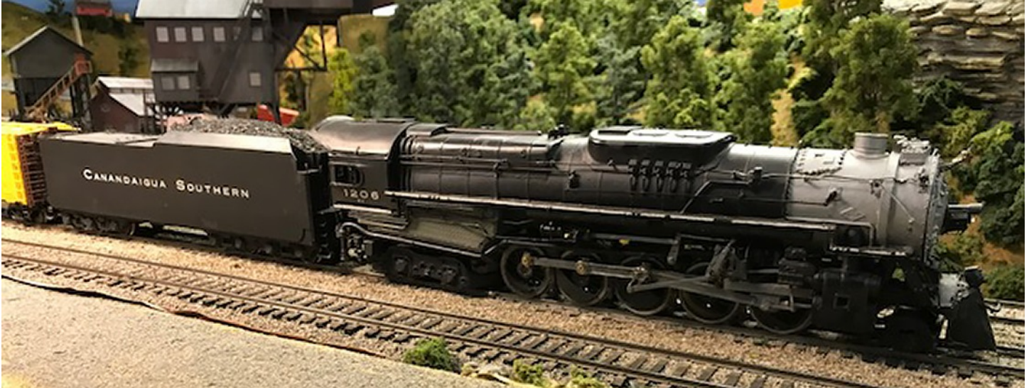
Photo 7A above: CSRR 1206 is a class V-1 2-10-4, one of 12 built for the railroad in 1944, using a variation of the PRR Class J design. CSRR made extensive use of belpaire fireboxes, a standard Pennsy feature, even though it had not been used on the Pennsy Js. The engine was customized by John Armstrong from a USH Pennsy J. It features the belpaire firebox the PRR would have liked but was not able to have. The tender is a stretched Lobaugh.
