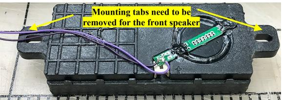
ACC on the connection so there would be no possible way they could touch, and then glued the wires to the speaker bottom. Double faced foam carpet tape will cover the bottom and secure to the tender chassis,
