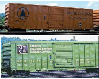
Included will be an FMC Boxcar center double door, FMC Boxcar diagonal double door, FMC Boxcar combination door and FMC 50'6" boxcars single 10' door. (Proto images shown)
