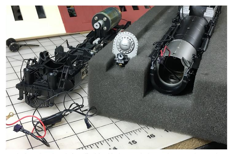
The picture above shows the front off and the wiring harness and voltage regulator out. We have to make some decisions here. The locomotive has a 6V bulb for the headlight and one LED in each of the class lights. The lights will come on at about 5 volts DC. With DCC they will come on and the regulator will supply the
