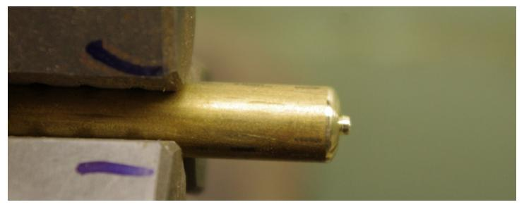
After I had the large radius on the end cut, I finished it with a file to make the small radius. This was much simpler than grinding a tool to do this in one cut. I turned the outside diameter to fit the tube, and cut the ends off the rod. When you cut the ends off the rod, make sure they are all the same. Drill the wire hole in the bung at this time, it's much easier now than doing it later.
