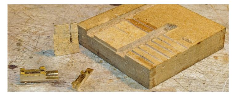
When all the machine work is done, pry the brass parts off the wood. Some of the wood will come with the brass. Drop the brass parts in some acetone for a while to dissolve the ACC glue. I have found this to be a good way to hold small parts for milling. You can also start to see the parts take shape.
