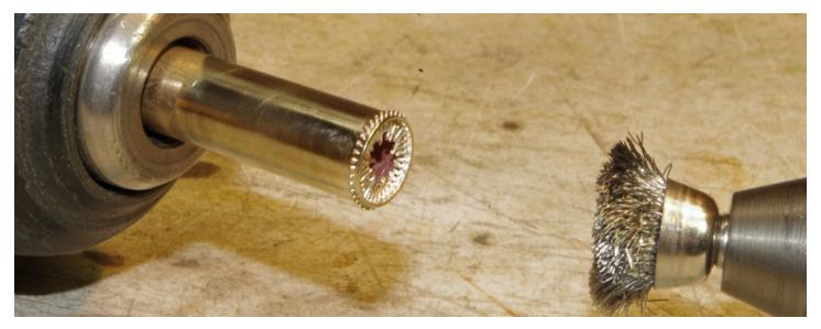
Look close at the previous photo, and you will notice the heads of the rivets are flat. They need to be softened up a bit. I did that with a wire brush in the motor tool. Then, I put the tube in the battery drill and ran it slow while running the rotary tool on the pins. It rounded the pins off nicely. I used the rotary tool with a carbide burr to remove the excess pins on the inside. Go easy with the carbide burr. They tend to grab on an inside cut like this.
