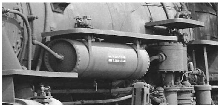
These are the air tanks I needed to make. Notice the brackets under the running board. I was rather surprised there was no saddle for the tank to fit in.
