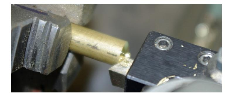
After I had the pins in the tubing, it was time to make the ends. I ground a lathe tool with an angle and hollow on it as shown, then ran it into the end of a brass rod. This was a simple grind to make and got me close. It gave me the large radius of the tank end and the bung for the pipe to thread into.
