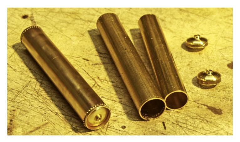
The tank on the left is done. The idea was to put the short tube inside the long one so it became a stop for the ends. In order to get the ends and short tube into the large tube, I needed to grind the pins flush on the inside. On the real tank, the rivets had heads on the inside, but I have not yet figured out a good way of doing that. This will have to do for now.
