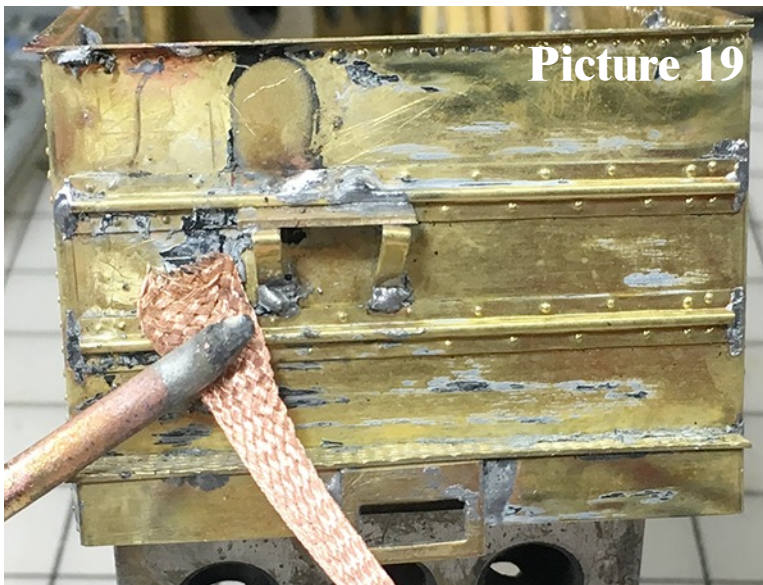
Picture 19 shows the cleaning of the old solder using a wick. The rest was filed down.
