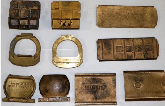
With respect to tenders; the following series of pictures show A&S castings for a Vanderbuilt tender. The first picture (left) shows two sets of the castings so that you can see both the front and the back of them. Note that not all of their castings are marked as A&S.
