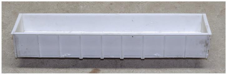
The basic body is put together. I used epoxy for glue because I wanted the extra strength and the gap filling properties. When you are clamping this all together, some glue is going to squeeze out. I use lacquer thinner and a stiff brush for clean up before the glue dries, making final clean up easier. When you are fitting the frame assembly, take your time fitting it and make sure the ends and sides that are not glued will line up.
