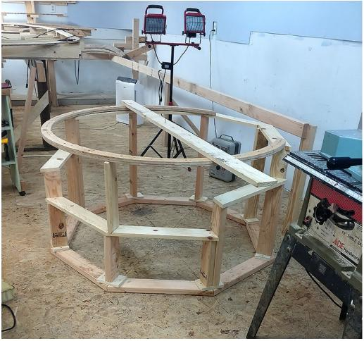
This substructure for Scalp Mountain was first designed on paper to get all the angles right, and then the parts were mass produced for quick and easy assembly.
