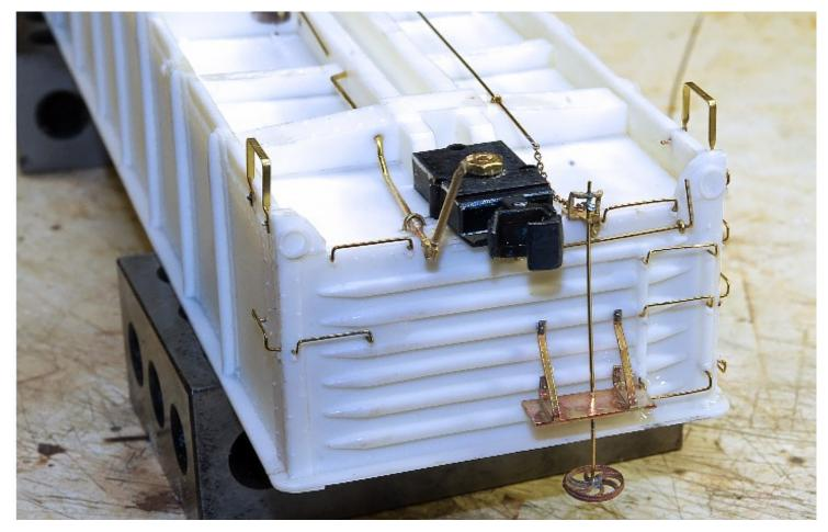
The end of the car put together. Notice the 2-56 nut holding the coupler on, a good secure connection yet easily removable. The steps and brake platform have brass nut bolt detail soldered into them. These act as pins and make a stronger glue joint to the resin material. The air line is held in place by a piece of wire bent over and inserted into holes drilled into the resin. I use gap filling ACC for these applications and get good results.
