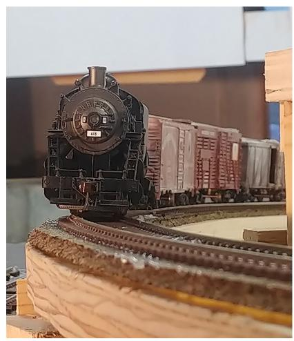
The first train on the Gorre Northern coming up the grade from Port on super-elevated curve. Track is Atlas glued to cork roadbed with clear silicone caulk.
