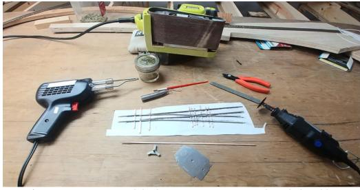
My first attempt at a scratch built turnout. Necessary tools include solderingscenes. His true to lifeiron, files, rail nippers, track gauges, and a belt sander to file down the frog andlighting system was designedpoints pieces. The turnout actually works!with his camera and specific
