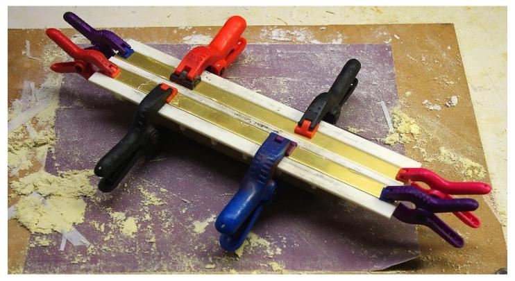
As I mentioned before, this kit has a thin overlay to the frame casting so there is detail on the car floor. The frame casting is rather thick on this kit also. I decided to add weight to the car by cutting some slots in the frame casting and gluing some brass bars into the slots. The slots were cut on the table saw and glued in with epoxy.
