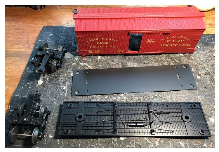
The car had nice doors that open and close, so I decided to add some detail inside. I created the illusion of bracing with strip wood. I drew pencil lines on manila folder cardstock to represent the half walls used on the inside of period wood cars. Some paint and dull coat finished the floor and interior.
