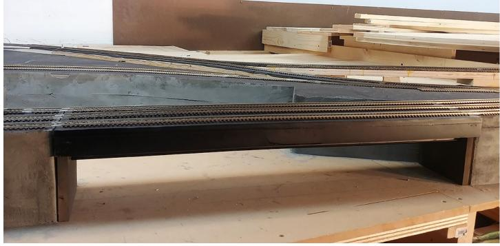
Temporary bridge over the harbor entrance at Port. It's made from a 1 x 4 board, 3/16 foamcore, scrap extruded aluminum for girders, all spray painted flat black. My goal is to get the pike fully operational right away, and there are scores of bridges to build for the completed layout. There will be temporary stand-ins for all of them...like this mock-up.
