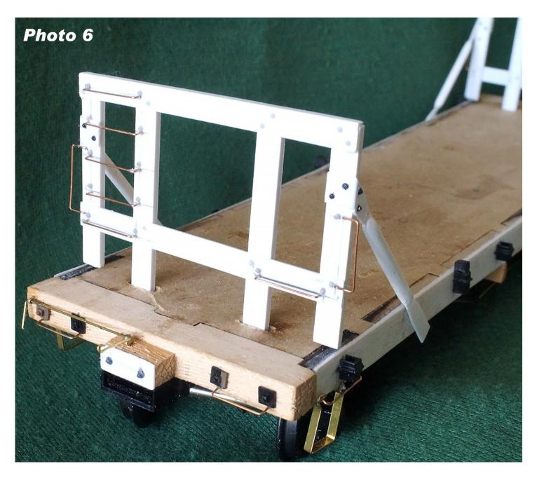
Brake wheel detail; which includes the brake wheel, staff, ratchet and pawl; was made and will be installed as a unit after deck is in place. On the prototype, the brake staff passed through the heavy end sill to a bottom bracket below the sill. A bracket was added below the sill for this.
