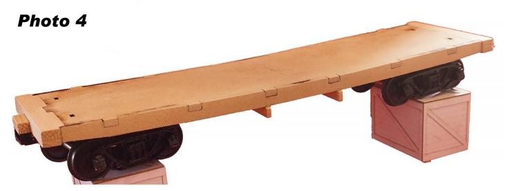
I cut strips of 0.20 thick styrene from a sheet and sanded the car frame sag on the top and bottom edges, "weathered" the outside surface adding wood grain by dragging my Zona saw over it, cut and sanded the end tapers to match the ends of the MDF side sills. The completed strips where then glued to the MDF side sills using epoxy. This covered the notches where the false floor interconnected with the bowed side sills quite nicely.
