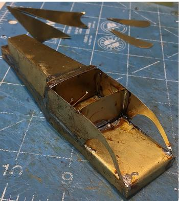
Step 4 the model is coming together. A little more cutting, fitting, filing, and soldering; then ready for clean up, more filing, filling gaps with body putty (50/50 solder) and getting ready for paint.
