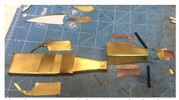
Step 2 was to cut out the brass pieces, bend to shape, and start soldering parts together.
