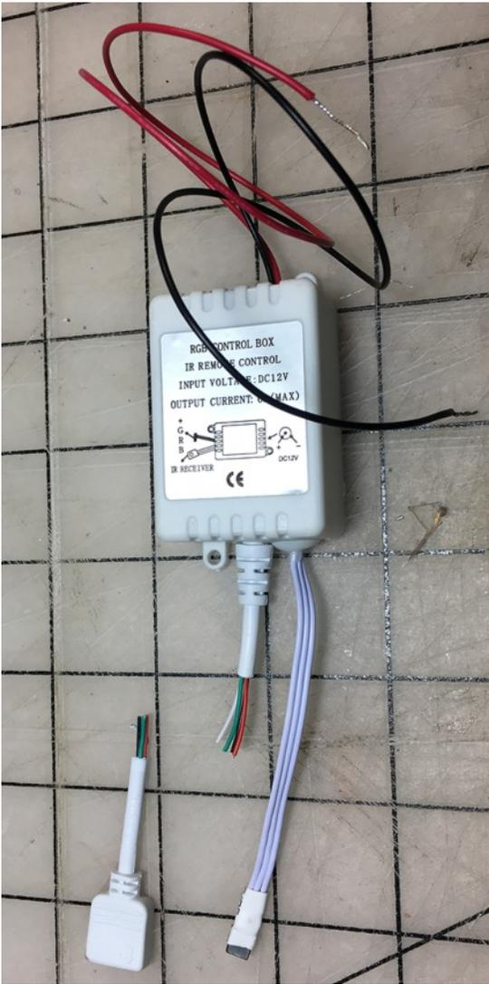
turned green. I pushed the green button and they turned blue. Red was red. This will be common between manufacturers. Mistakes can and do happen. Simply swap the wires going into the amp that control the blue and green. Trust me here, do all your testing on the bench because plugging in the next amp and LED string, the colors could be off again. Easy fix, but easier on the bench.
