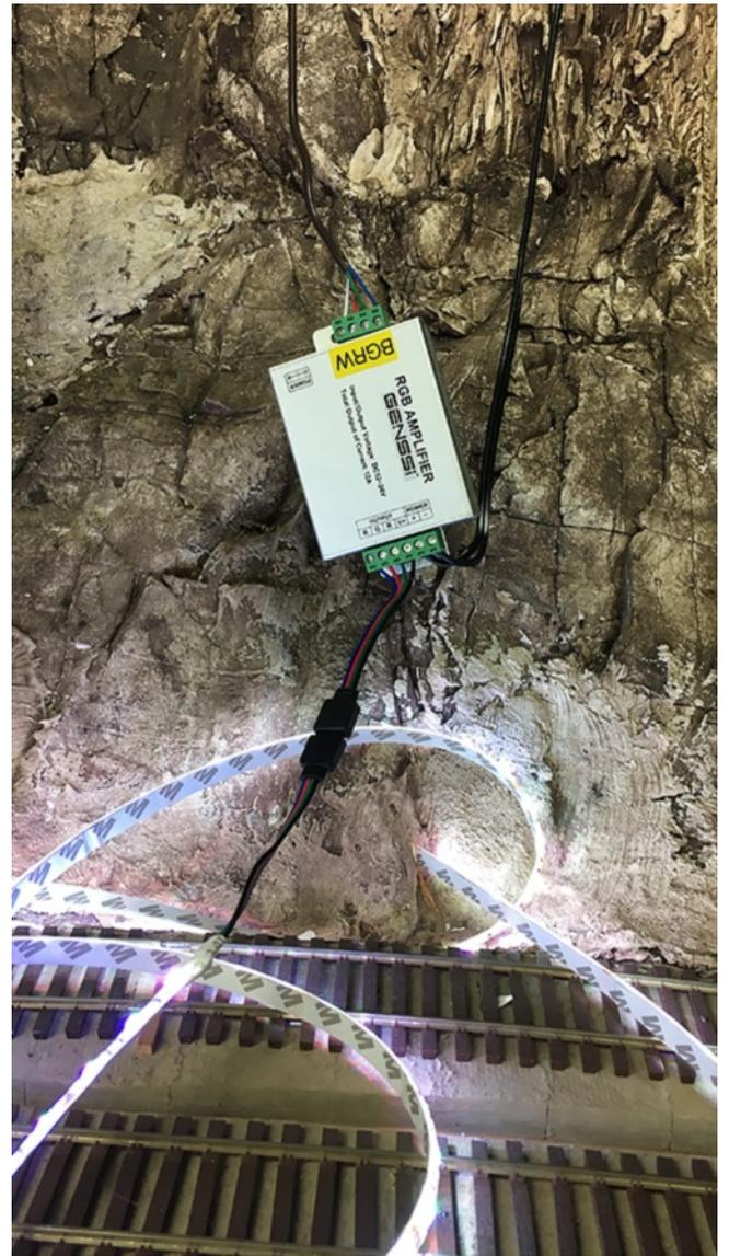
Below: Installed on floor joist. The four wire cable in on the right coming from the control box that was mounted under the layout. On the left side, the black lamp cord brings the 12 volts up and the four colored wires connect to the first full LED string. This is amplifier number one. See drawing on next page.
