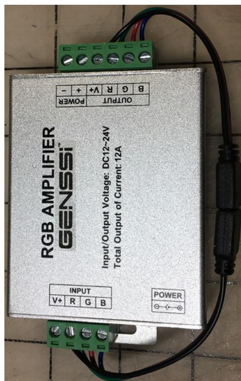
The RBG amplifier is used when more than one LED string is tied together. I figured this out the hard way as you will learn. This also needs a 12 volt source.
