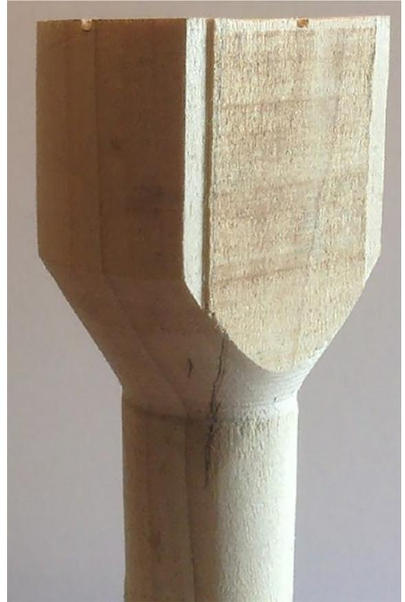
*Divider flat cut, with rivet flange relief.*
