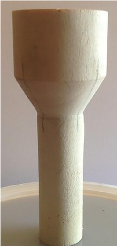
*Mold for pots turned on lathe.*
