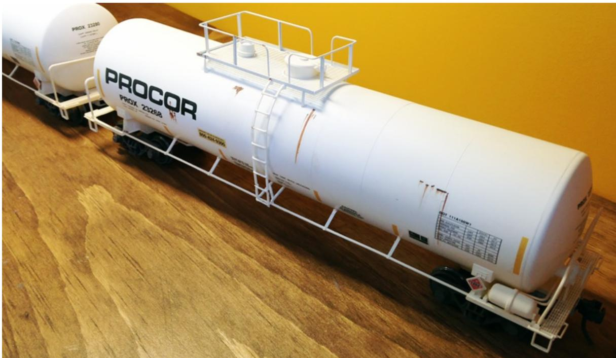
*I love to buy old cars for a few dollars and re-build them. Here is a good example. This is a Weaver tank car which I added weights and glued the body so I could fill all the seams. I also scratch built a new platform out of photoetched brass and florists wire for the handrails. I then printed the decals on my Alps printer and applied a very light weathering to the car and trucks, which are old Athearn trucks with Intermountain metal wheels.*
