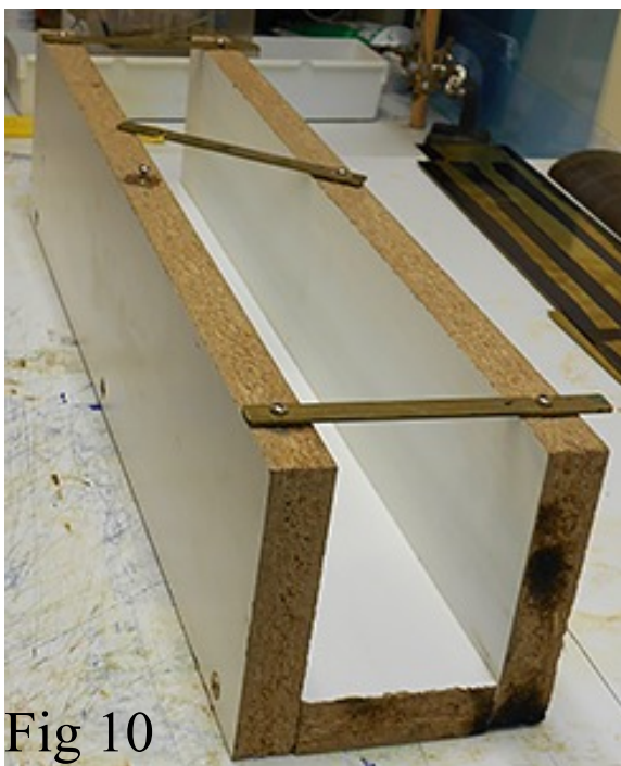
Figure 10 – Assembly fixture with clamps that lock and hold everything tight.
