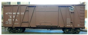
The second car is also SP, class A50-5, a 50' end door auto car, also singled sheathed. model built by Paul Hecht. Both cars built in the 1920's and ran into the 1950's. Both models have end doors for loading long bulky items, like roof trusses, machinery, fire engines and other products. SP subsidiary TN&O also had some of these classes.
