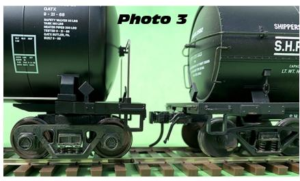
The model measures 39 ft. long by 9 ft. 6 inches wide. Overall, the model compares well to an Atlas O 11,000 gallon tank car except for the **too high bolster height.**
