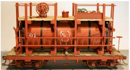
Water Wagon. Morgan Hill Models wood tank car freelance bash of a fire train water tank car.
