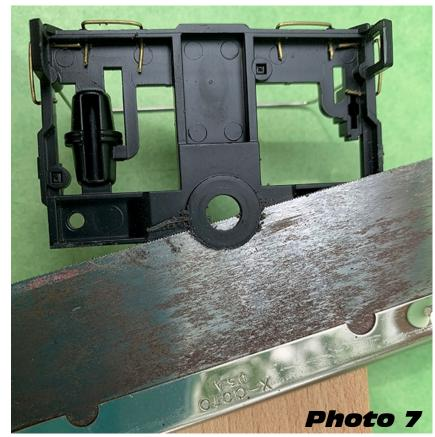
Photo 7: Underside of plastic end frame. Remove plastic boss with X-acto saw. Caution: do not remove this boss until you have used its hole to locate the new hole in the new centering plates. After removing the boss, the remaining hole is enlarged to receive the large boss on the truck. The rectangular cavity in the frame will be filled in with styrene to create a pad to mount our new Kadee couplers. New brass grab irons installed.
