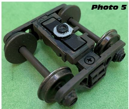
Photo 5: Finished upgraded truck. 3-rail wheels replaced with InterMountain scale wheel sets. The axles, wheel faces and side frames have been painted a dirty brown. 3-rail coupler removed and extra appendages cut off bolster center section. Top side of truck bolster has large boss painted light gray to show clearly in the photo. The smaller boss shows up well too.
