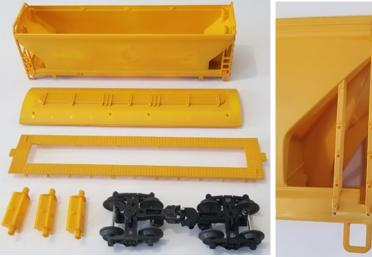
I will not make this entire article about how I modified these cars, but in short, what I did was to remove and discard the roofwalk, the hopper gates and the trucks, and cut-off all the ladders and grab irons. I then drilled holes and created new ladders and grab irons out of brass rods.
