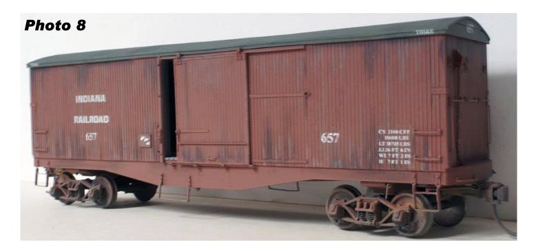
overlays are used for the side sills; and thick, .040 inch thick scribed sheet used for the car siding. Any required rivet detail can be pressed into the thin styrene side sill overlays before they are installed on the model, or they can be added using decal rivets at any time.
