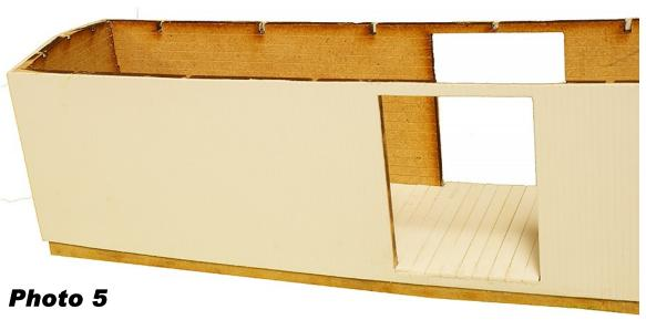
Another nice feature made easy by this approach is building a scale car roof. Again, from the photos of IRP 201, you can see notches 1/16 inch wide cut into the subsides and sub ends into which styrene carlins and purlins, to support the roof, are placed. And, Photo 6 shows the carlins and
