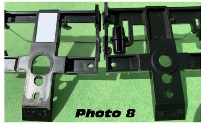
Photo 8: On left, bottom side of plastic end frame with boss removed. Center hole has been enlarged and shaped. New styrene pads fill in the rectangular cavity in the frame for mounting Kadee 805 couplers. Unmodified factory end frame on right.
