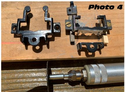
Photo 4: Remove the extra 3-rail coupler appendages no longer needed. On the right, the truck's center section is securely held down with brass wood screws while being cut with a Dremel rotary cut-off disc. O scale wood ties support the pressure of the screws to prevent bending or breaking the tabs.
