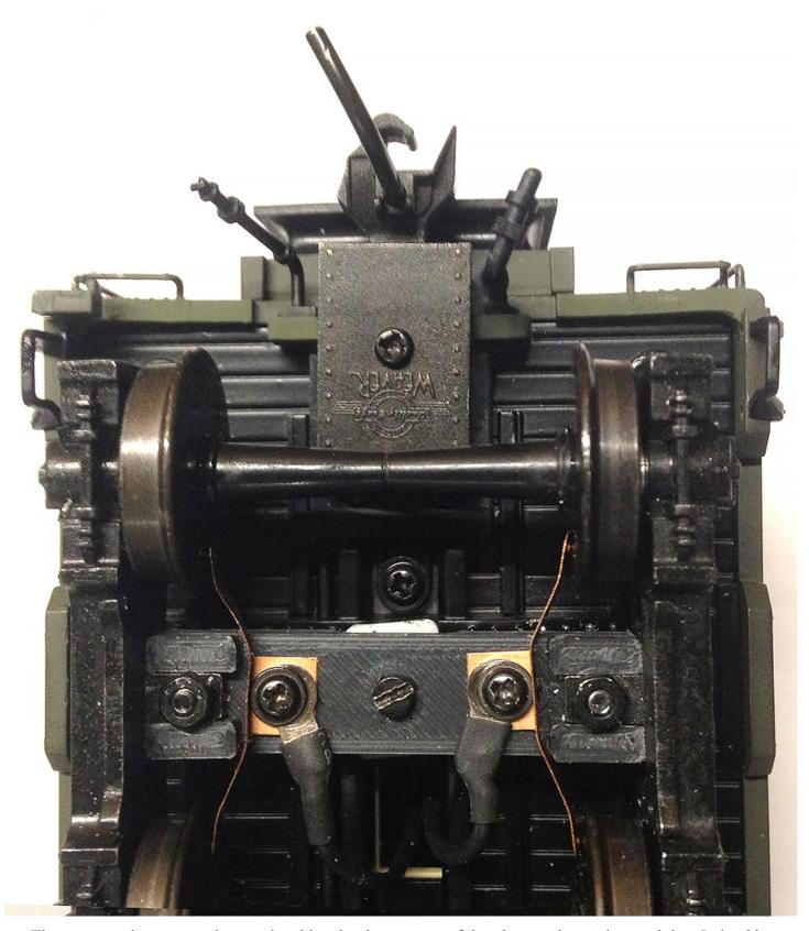
The next step is to screw the coupler shims in place on top of that the coupler pocket, and then I glued in either top corner the plate with the steam and air connector. After this is dry, the car is ready for a test run. What I didn't do was to replace the coupler centering spring with a piece of plastic tube.
