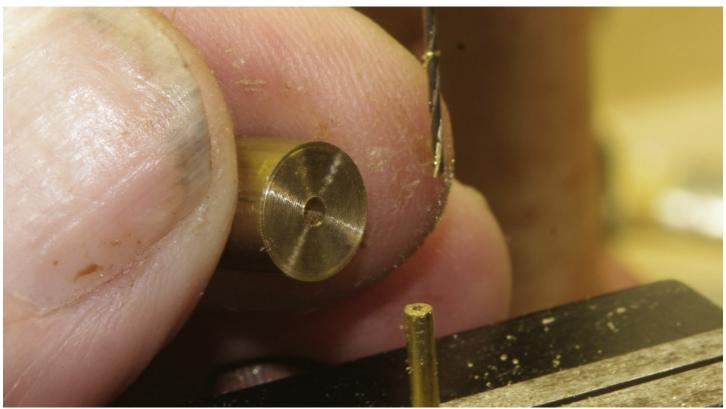
This will give you a better idea of how I drilled a hole in the end of some .062" diameter wire. I drilled a .062" diameter hole about .125" deep in the brass while it was in the lathe. Then, before removing it from the lathe, I drilled a .025" hole deeper. Now I have two holes that are concentric. Place the larger brass piece over the end of the wire and drill the .025" diameter hole using the brass as a guide.
