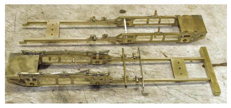
Here is another photo of the frames. The top frame has the blocks that I used to space the driver bearings when setting up the spring rigging. The bottom frame has the cross head hanger and pilot beam in place, but not soldered yet. So far so good.
