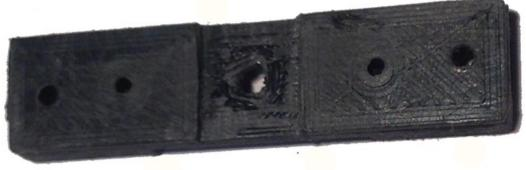
The new bolster. The square for the distance piece has been narrowed to 8mm.
