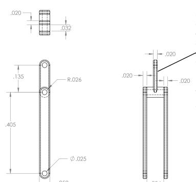
This top link would be difficult to make as one piece like it is drawn. I decided to make a flat link and solder a bushing on each side. The long links, bushing and top links would be pinned and then soldered together as a unit. That worked.
