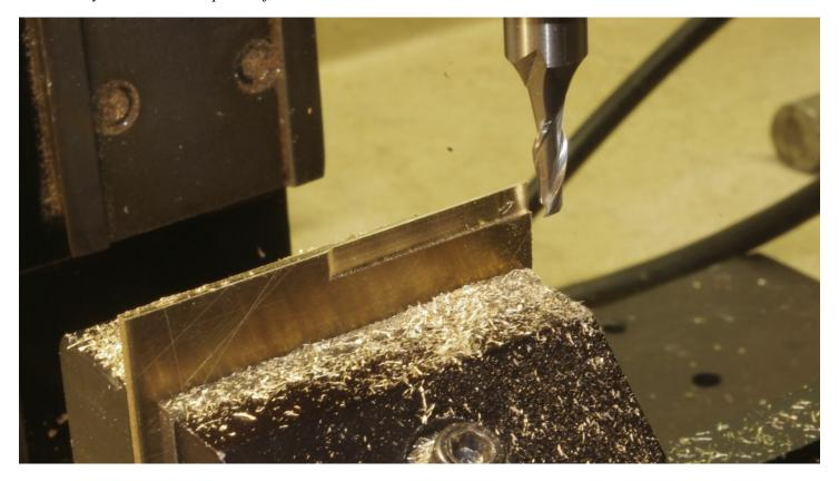
Part of the spring rigging had a small "T" shaped piece. I put a piece of brass plate in the vise as shown and cut on each side of it as shown. After this, I cut off a piece of this for the next operation which is in the next photo. You will get the idea when you look at that photo.
