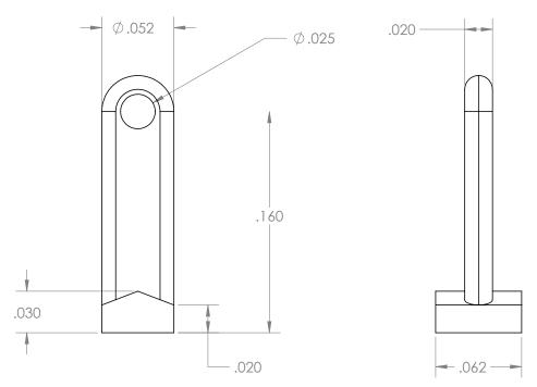
This hanger goes through the equalizer and through the spring. Look close at the dimensions. I needed 8 of these. By using the "loaf of baloney" method I was able to remove most of the material in one set up. Then I cut the loaf of baloney off the brass plate and cut the individual parts off the loaf of baloney. See the next 2 photos for how it worked.
