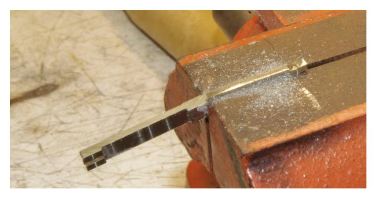
After I had the ends of the equalizers slotted, I just filed the taper in place. This worked fine. This is a feature that is for looks and not function.
