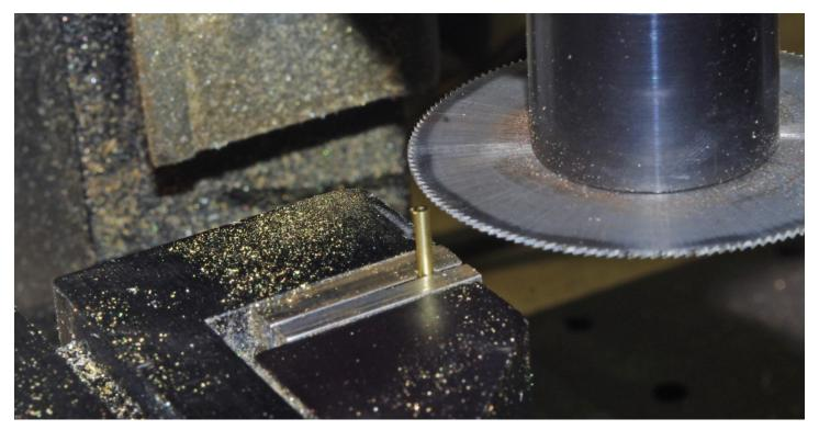
This is how I cut off the bushings. These bushings are .062" diameter and .030" long. The .010" thick slotting saw made quick, accurate work out of this.
