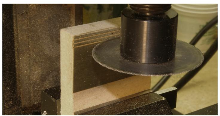
I needed some .052" X .020" brass strip and had to make my own. This is the set up I use for cutting strips. Cut one line first and that will be your starting point. I am using the .010" slotting saw here. Don't forget to take into account the thickness of the saw. I wanted .052" wide strips so I needed to move the saw down .052" plus .010", for the saw thickness, or .062" total. Pop them off the wood and soak them in Acetone to clean them.
