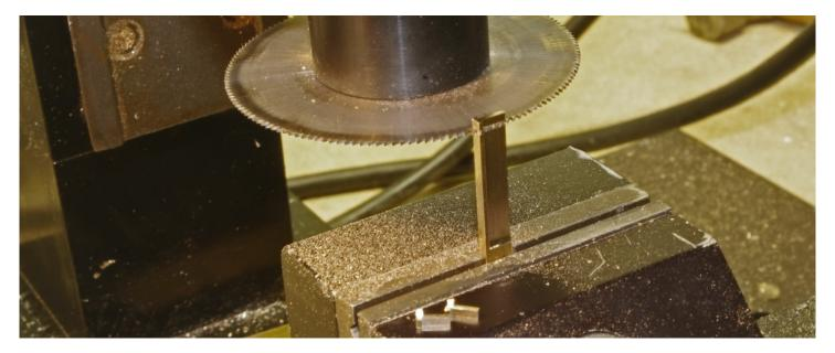
Here I am cutting off the parts. One of my machinist friends called this making a "loaf of baloney" and cutting the parts off. I have been doing a lot of this on these models. Look at how small the parts are. Can you imagine holding them to machine them? They also call this "leaving a handle on the part" I was able to hold the part tight in the vise with the "handle" and cut off the parts from the baloney.
