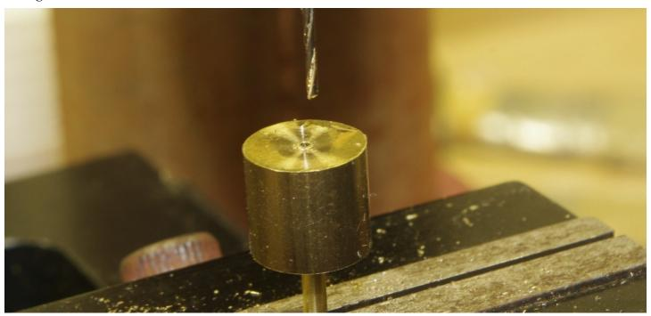
This is a simple set up I use for drilling a hole in the end of a piece of wire. I needed some .062" diameter bushings with a .025" hole in them. I started with some .062" diameter brass wire. My lathe will not hold wire this small. After doing this, I found I could turn a .052" diameter on the end of some .125" diameter brass. That would work better, but this set up is worth putting in the back of your mind. It may come in handy some day.
