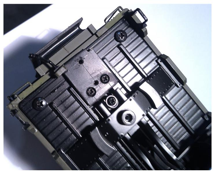
The new coupler shim. The cut outs for the air and steam lines are visible in the top corners. The 2 holes have 2mm threads to screw the coupler in place.
