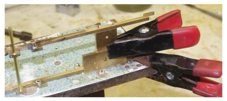
This is how I soldered the front of the frame under the cylinders together. Notice the pins again. I will file them off next.
