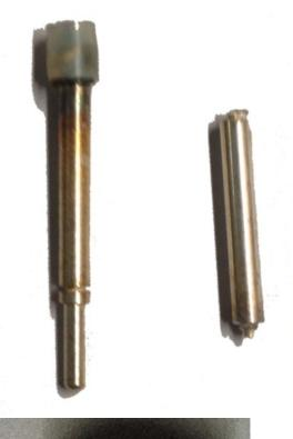
The pins that I used. The two cuts are for C-clips to secure it in an insulating nylon bushing. The short piece above is the remaining piece after cutting the pin at the recess off.
