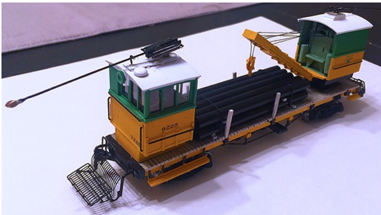
A scratch-built fully-operational HO scale model of Los Angeles Transit Lines' 9225 derrick. The crane is also motorized and DCC controlled to rotate on an independent control circuit from the main car drive.
