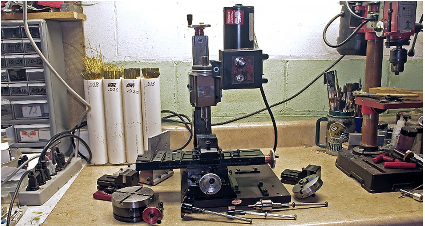
Sherline Products makes small precision machine tools. This is one of their vertical spindle milling machines and some of the accessories they make for it. Note the size of it on my work bench.
