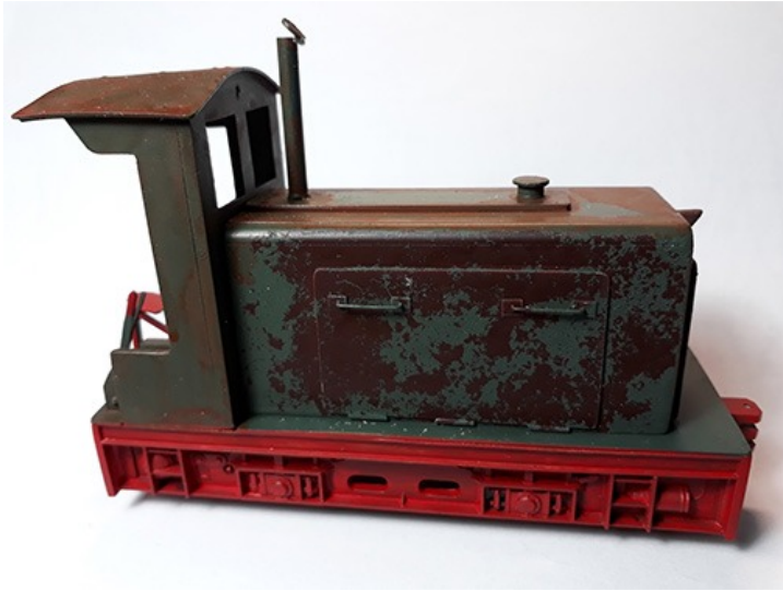
Industrial Diesel in 1/35 based on an HO Model Power Plymouth powered underframe. Cab and hood are scratchbuilt from plain styrene sheet.
