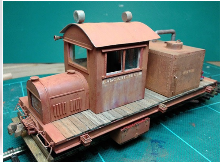
On30 M.A.C. Rail Car. Deck, cab, hood and tank scratchbuilt. Powered by a Bachmann HO Railbus.
