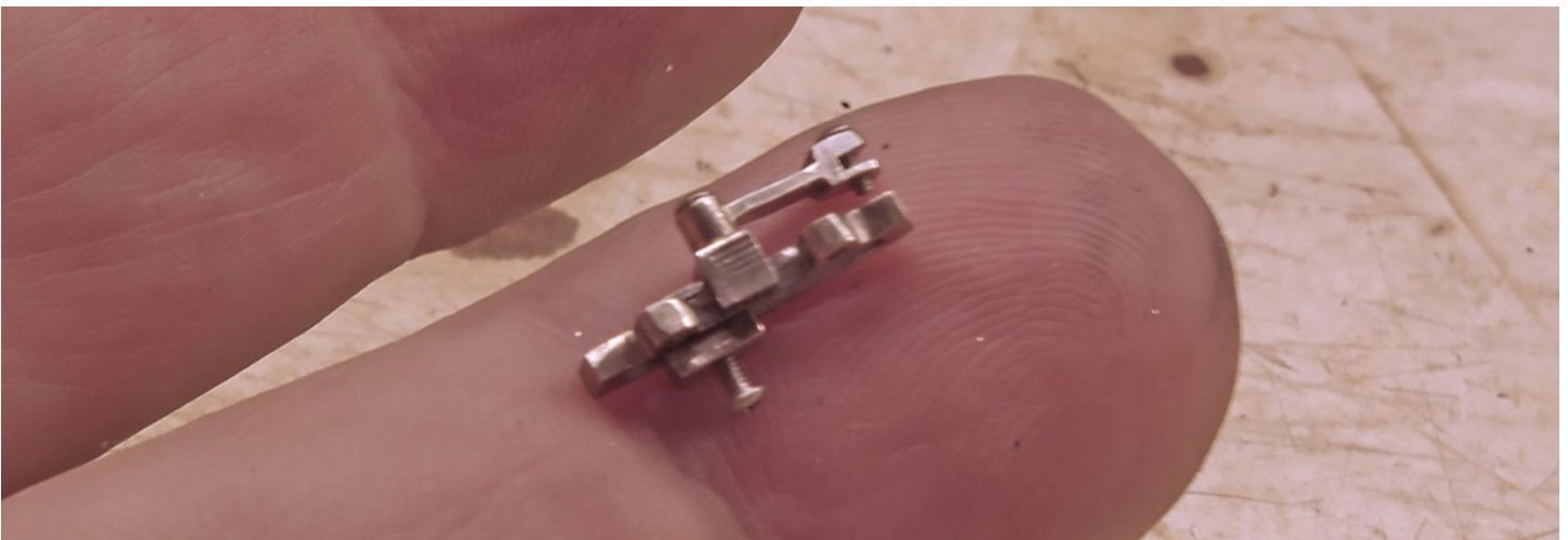
This is a finished link with the link block and hanger installed.
