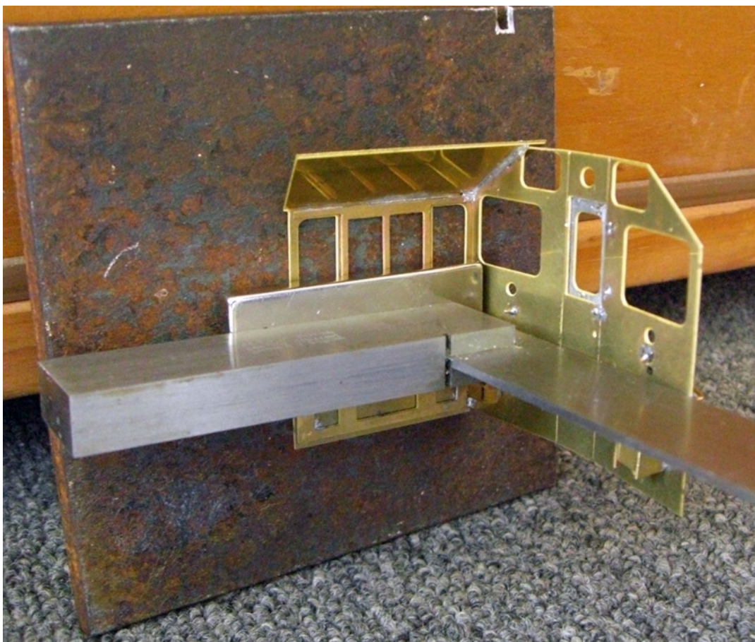
The 2"x1"/50mmx25mm shiny metal magnet is peeking from behind the handle of the engineer's square. The rear cab face rebate can be seen on the left below the square.
