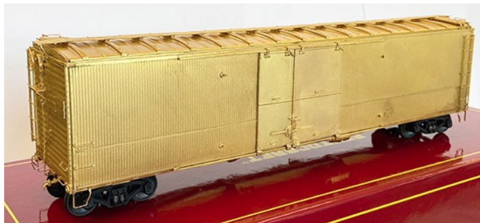
PC-3701a - Series 61200-61399 Has a unique Inverse Murphy end under a Chicago-Cleveland Climax Radial roof.
