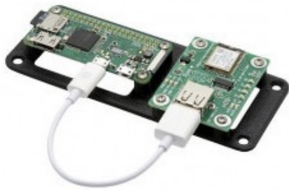
ProtoThrottle Receiver for ESU CabControl, JMRI WiFi Throttle, and Digitrax LNWI.
