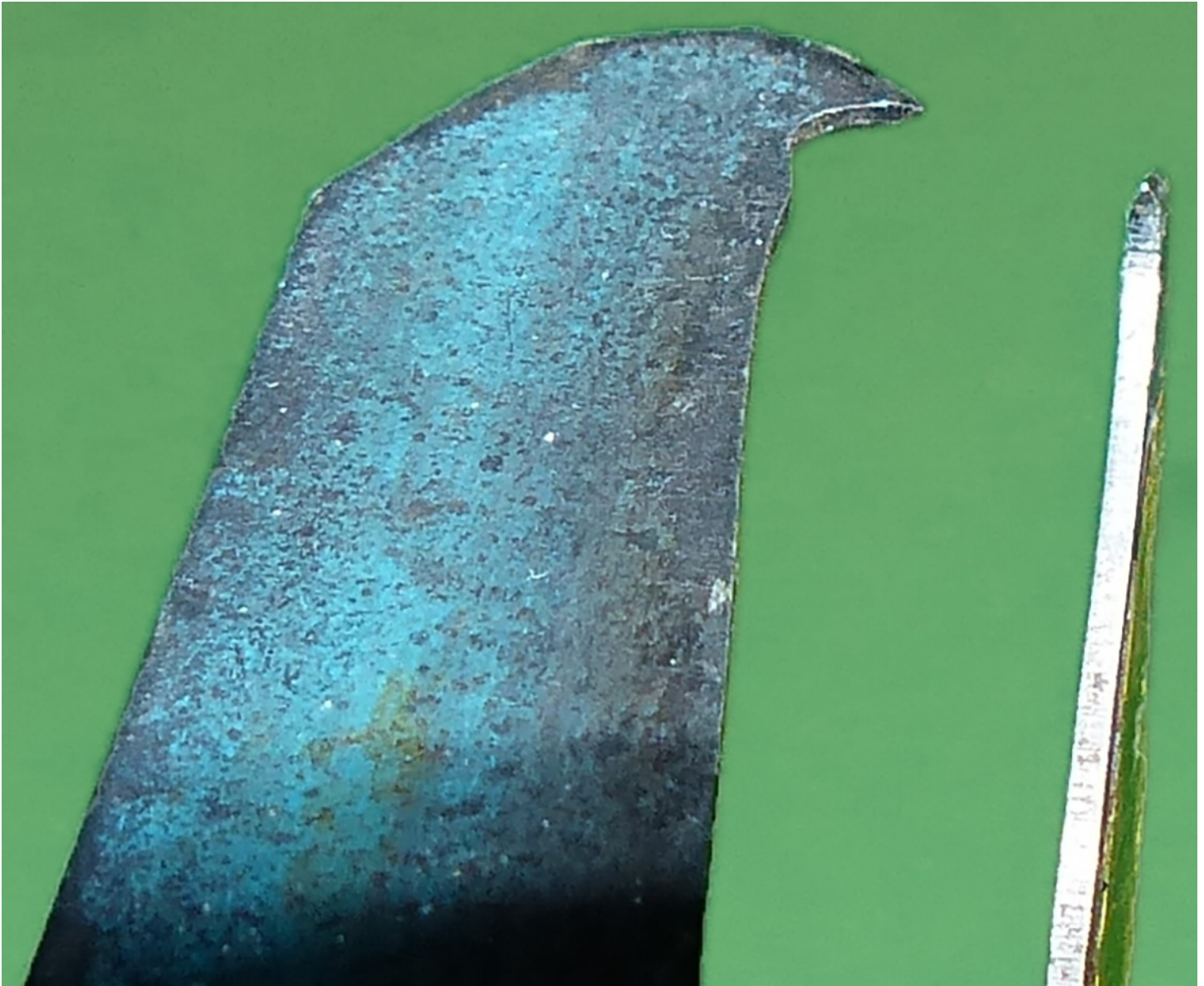
Scawker ground from broken hacksaw blade.
