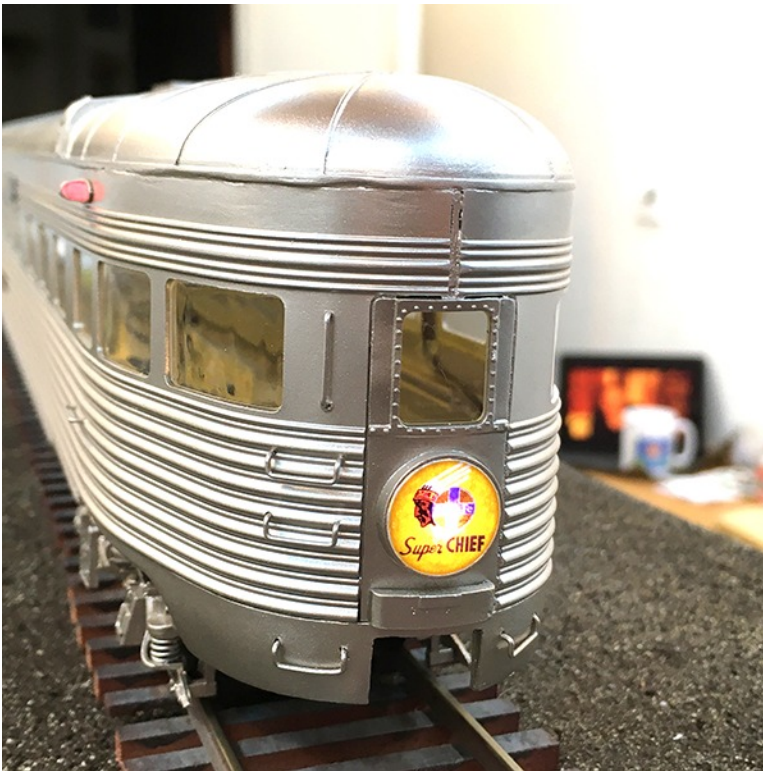
The drumhead looked so bright before modifying the LED, the letters on Santa Fe cross were illegible. The drumhead LED after a pass of a loaded brush with yellow stained-glass paint.
