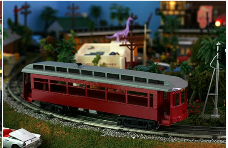
Passenger trolley – scratch built from balsa and styrene, power by an a 3 pole open frame motor and gear driven. Photo by author.
