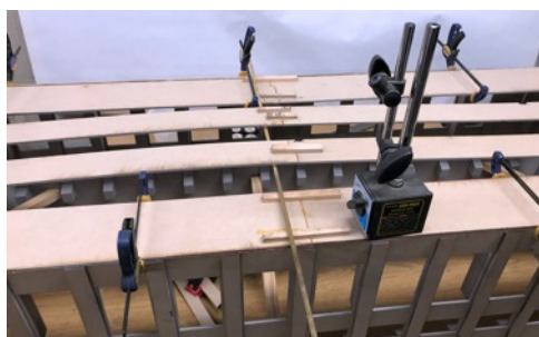
My method for reducing the sag in the center floor legs until the glue dried.
