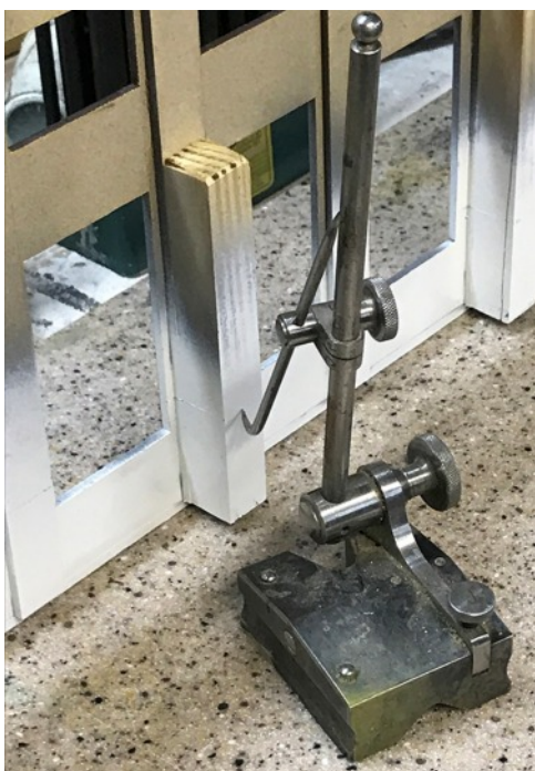
A Starrett surface gauge was supposed to engrave a level line around all the interior walls... that was until it was slipping during the process.
