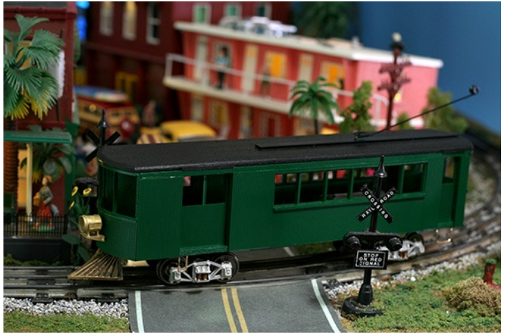
Combine trolley – scratch built from balsa and styrene, powered by an N20 motor and a rubber band drive. Photo by author.
