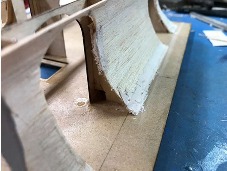
Above: Mansard roof skinning require additional fillers behind the skin flanking the window cuts. The balsa was very fragile.
