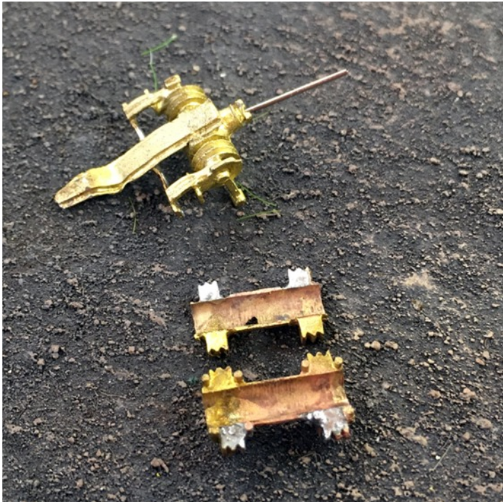
Once freed from the PSC trucks, these three pieces made for the Pullman drive components. The orange circles indicate the extensions that needed to be trimmed.
