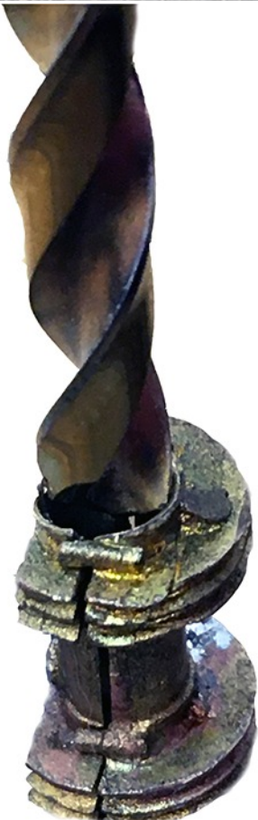
A 5.00 mm drill bit expanding the axle-mounted hole.
