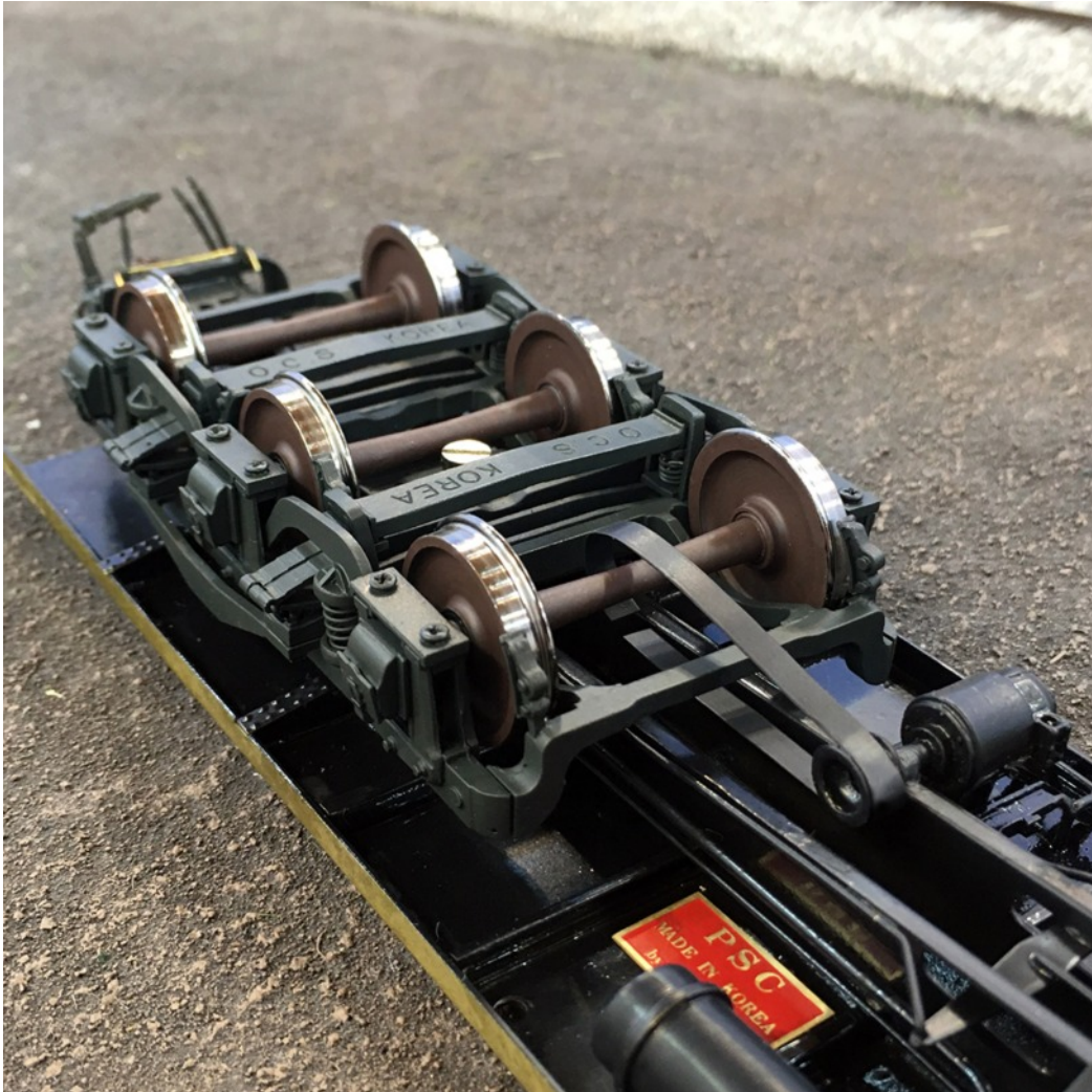
Close-ups of the final assembly. The Wasatch trucks further improve the already busy and plan-specific PSC undercarriage.
