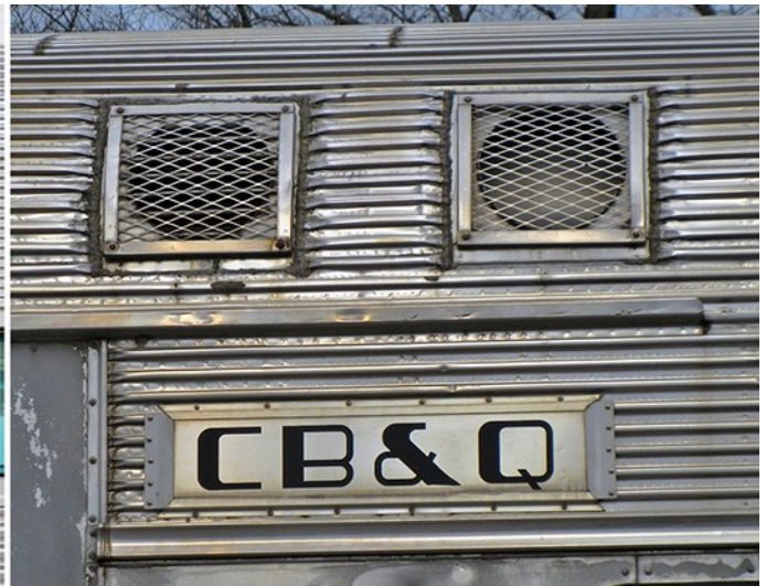
A close-up of the vents on the prototype reveals the screen that was used on the cars.
