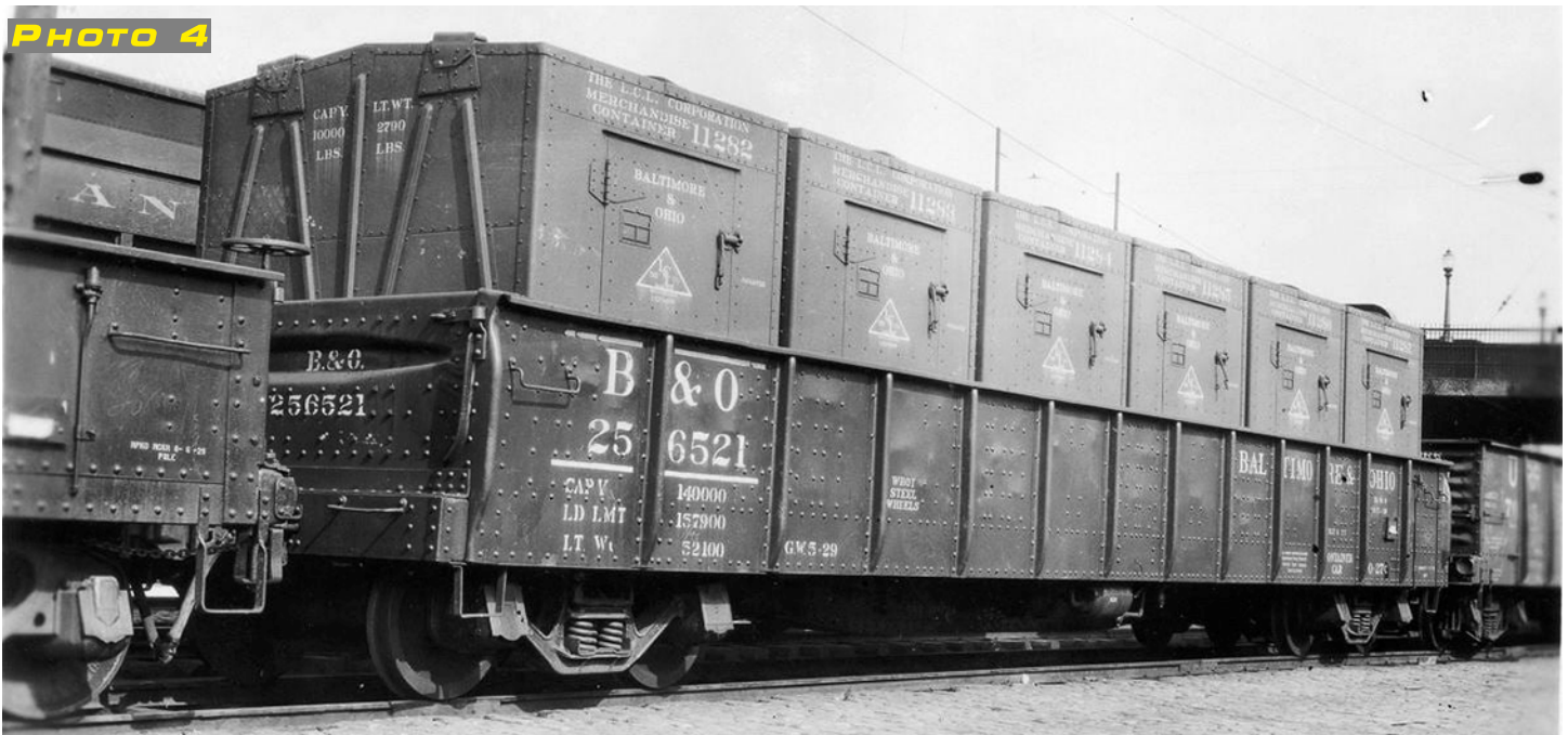
One enterprising firm, the LCL Corporation, provided several thousand containers for this traffic. Photo 4 shows a B&O gon loaded with the quasi-standard LCL Corporation merchandise containers.
