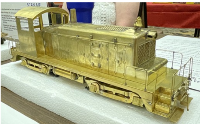
The hood of Glenn Guerra's brass SW-1 along with the air tank ends and headlights were just some of the parts Dan Dawdy printed for Glenn, who then did the wax molds that were cast in brass for the locomotive.
