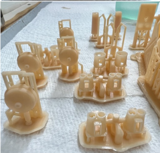
The hood of Glenn Guerra's brass SW-1 along with the air tank ends and headlights were just some of the parts Dan Dawdy printed for Glenn, who then did the wax molds that were cast in brass for the locomotive.
