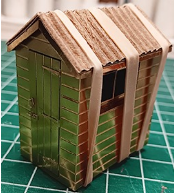
Aleene's Tacky Glue spread over the brass subroof and a couple of rubber bands kept the steel in place until the entire assembly dried.
