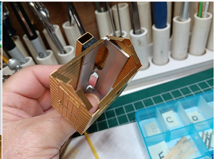
After folding the four walls of the shed together I used my Coffman "Original Right Clamp" to keep the corners square and tight for gluing.
