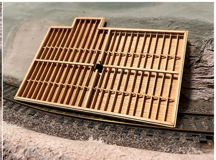
This is the underside view of the floor showing all of the floor joists and cross-bracing. The bracing is made from a file card cut in thin strips and there are 96 of them.
