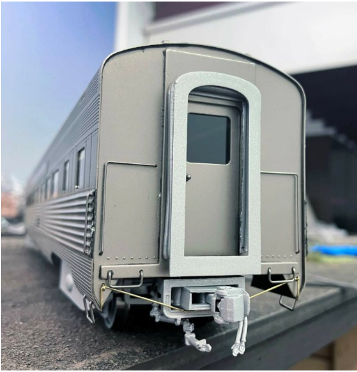
The attached coupler cut bars before paint. The finished diaphragms were already in place.
