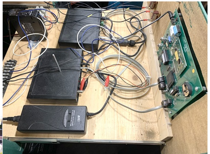
Photo 17. The components of the Easy DCC system are stored in a drawer for easy access and to keep them clean.
