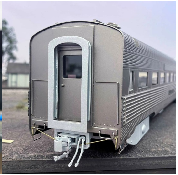
The attached coupler cut bars before paint. The finished diaphragms were already in place.
