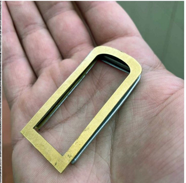
The laser cut round style diaphragm plate with the added accordion rubber.
