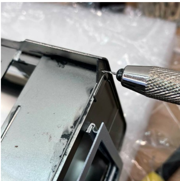
Left: Drilling the holes for the cut bar brackets. The coupler cut bars were made out of .020 brass
