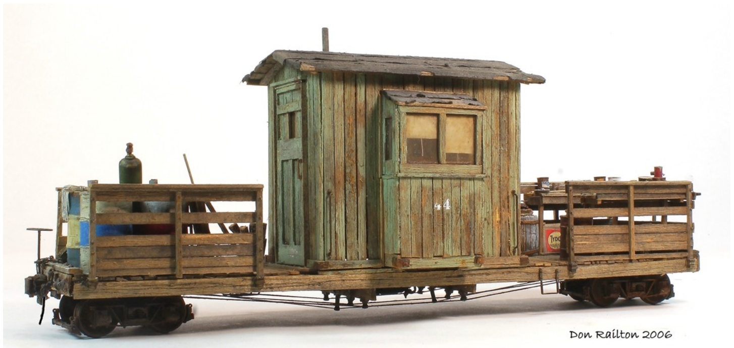
Green Caboose - A narrow gauge work caboose from scratch using San Juan Car Co. trucks and brake system.
