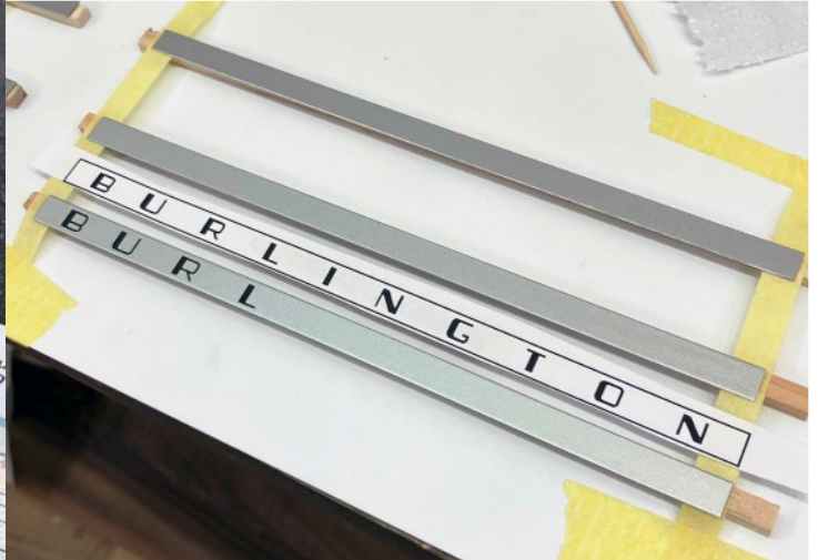
To ensure the individual letters were neatly placed, a printed template guided the application.
