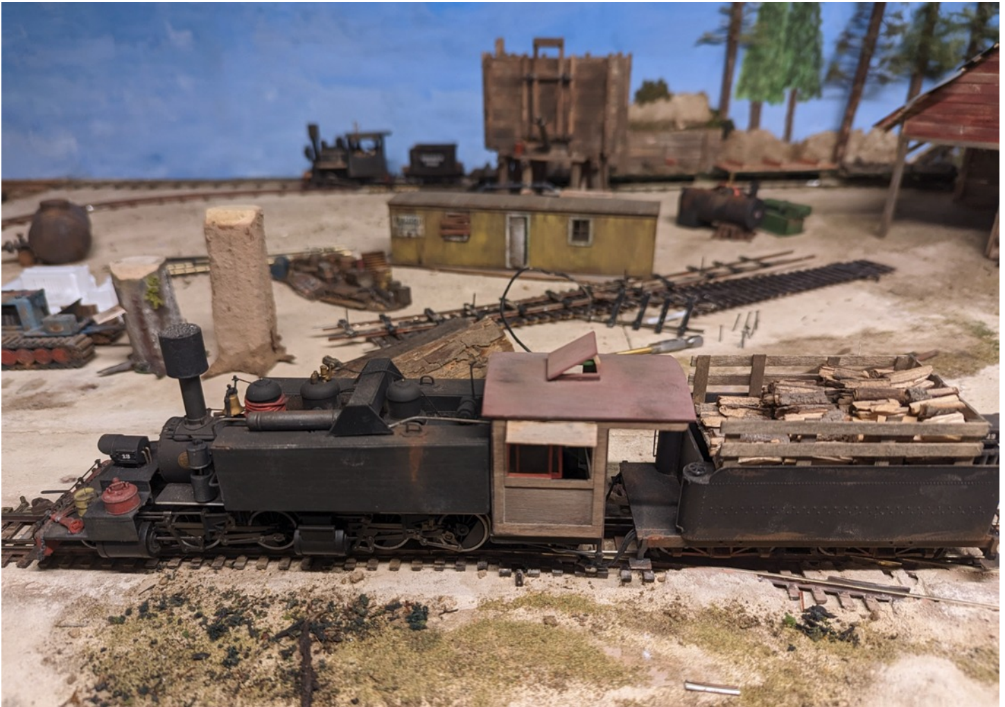
This is my 2-4-4-2, my original foray into kitbashing. I made the side tanks out of styrene and 3D printed the pilot for the loco. My biggest risk was relocating the headlight to the pilot off of the boiler. It worked out well. It gave me the confidence to move the headlight on a Shay later. This loco resides on Joel Bingham's On30 Sespe Western.
