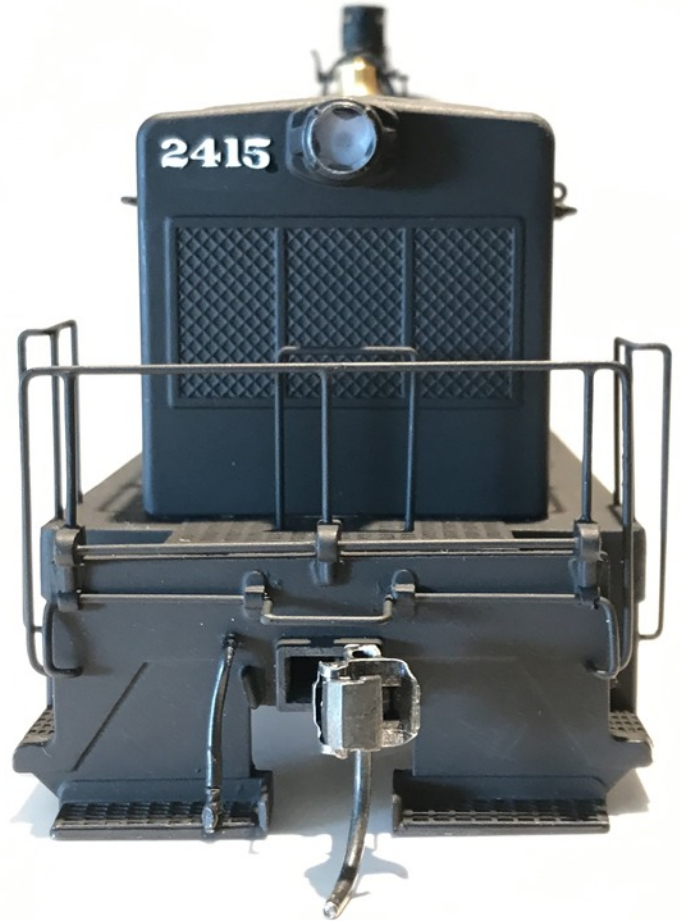
3D printed engine numbers with alignment sprue and finished numbers with single MU hose in proper position on front pilot.
