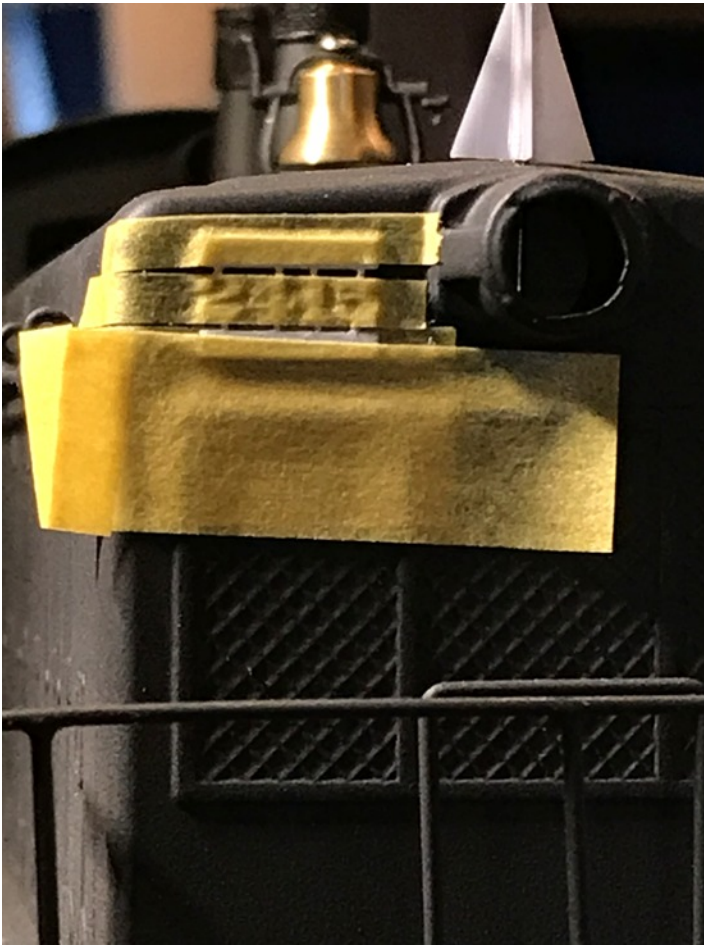
3D printed engine numbers with alignment sprue and finished numbers with single MU hose in proper position on front pilot.
