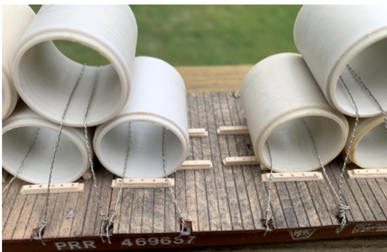
The years old resurrected wood and metal castings Quality Craft PRR F-41a bulkhead flatcar ready for duty. A few minor repairs, the trucks and couplers cleaned and made road worthy. To complete the resurrection, the wood deck and bulkhead boards were cleaned with a soft wire brush and then re-stained with dirty brush cleaning solvent.
