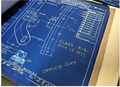
When railroads bought new equipment they usually got a complete set of drawings from the manufacturer. This example is an American Locomotive Company drawing of a part for a C&NW class E-4 Hudson type. This is an original ALCO drawing, but many times the railroad would trace the manufacturer's drawings. For example the title block would say C&NW but the margin of the drawing would have a notation that it was traced from a manufacturer's drawing.
