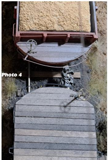
one of our passenger cars. Passenger cars tend to run in trains together and are not coupled and uncoupled all that often. These Wagners work well and are of a tight-lock style with no tendency to jack-knife. But using these dummies on freight cars was not the answer. For one thing, they are closer to a very small prototype knuckle coupler than Kadees, and do not couple well with Kadees. And, the Wagner couplers are now hard to find as they are no longer made.
