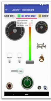
prototypical operation and consist on the fly. It features real time scale speed display and haptic controls like vibration for each throttle notch or pressure-sensitive emergency stop.
