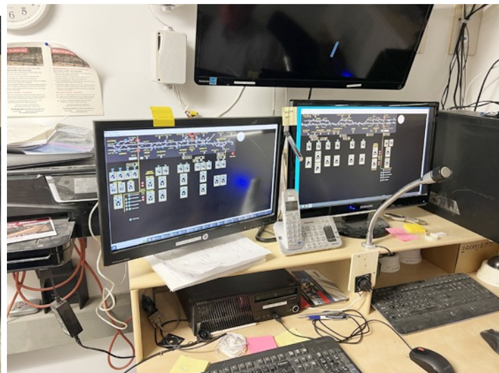
CTC Dispatcher panels for the Central Ontario's 8 scale mile long mainline. Created using JMRI software allowing prototypic traffic control by signal indication according to Canadian Railway Operating Rules c.1962
