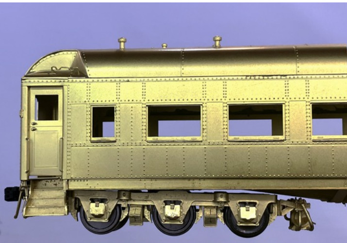
Holding the car up in the air, the trucks no longer dangle thanks to the new truck screw.
