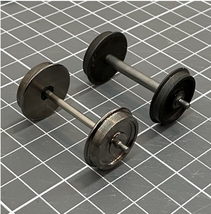
The GGD wheels to the left and the PRB wheels on the right. The GGD set fits the bearings, and their reflective appearance is more prototypical.
