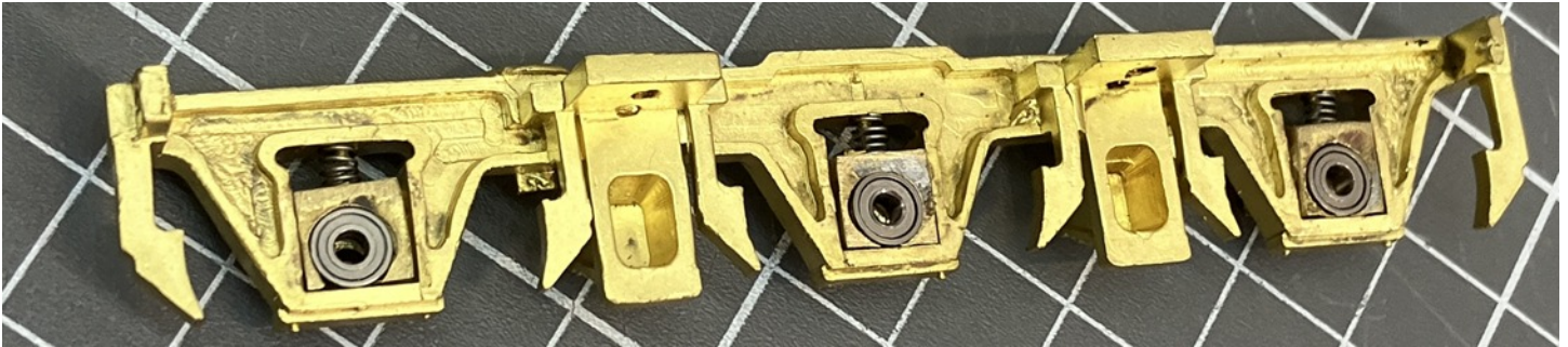
The reinstalled journals with bearings. The sides of the journals were filed to ensure a slight play for proper equalization during operation.
