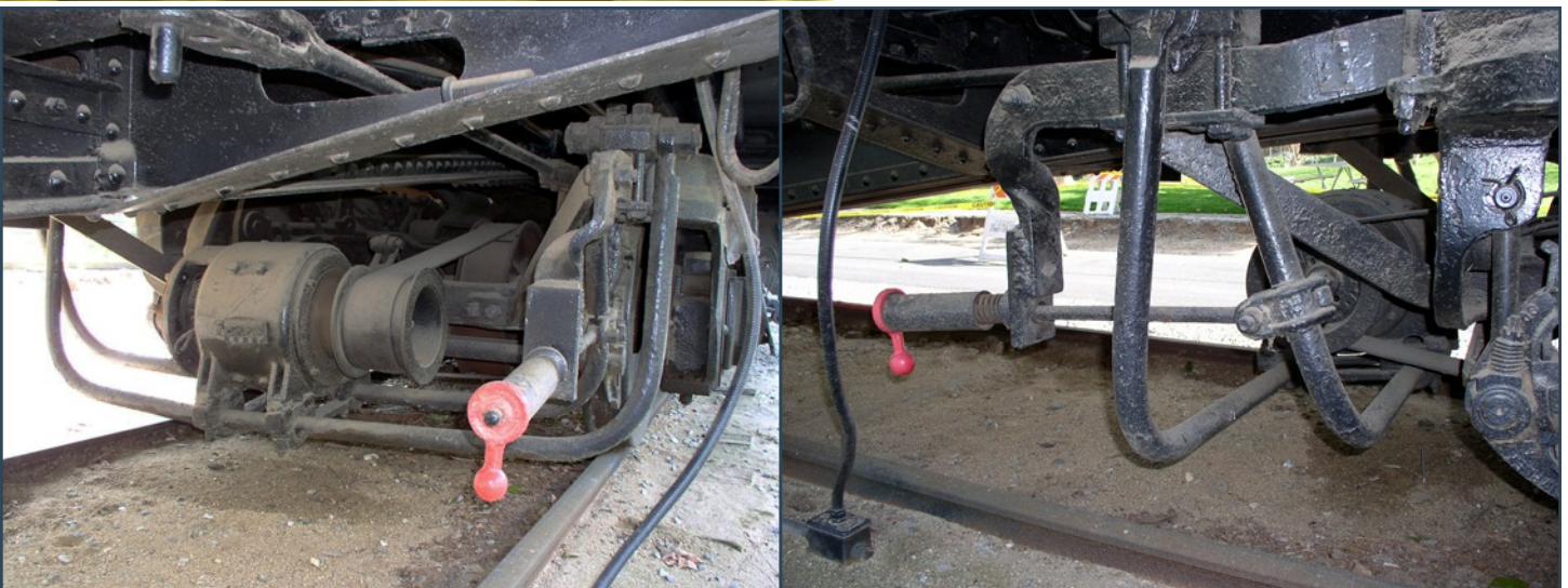
On the AT&SF heavyweight cars, the truck mounted generator belt was openly visible. To simulate the rubber material, the copper strip will be painted matte black.
