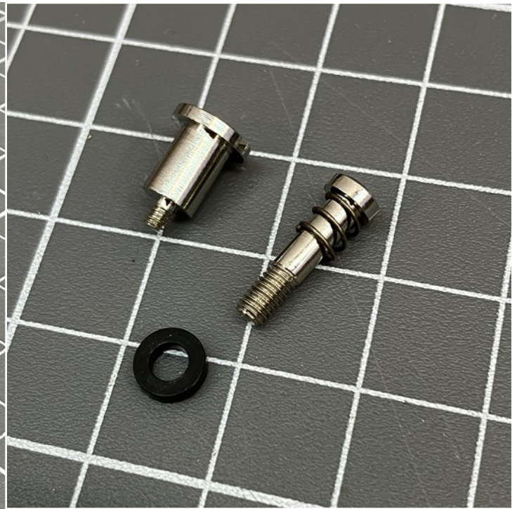
The PRB 1.5mm screw on the left, and the 2.5mm screw on the right. The black bushing keeps the springs from going through the plates.
