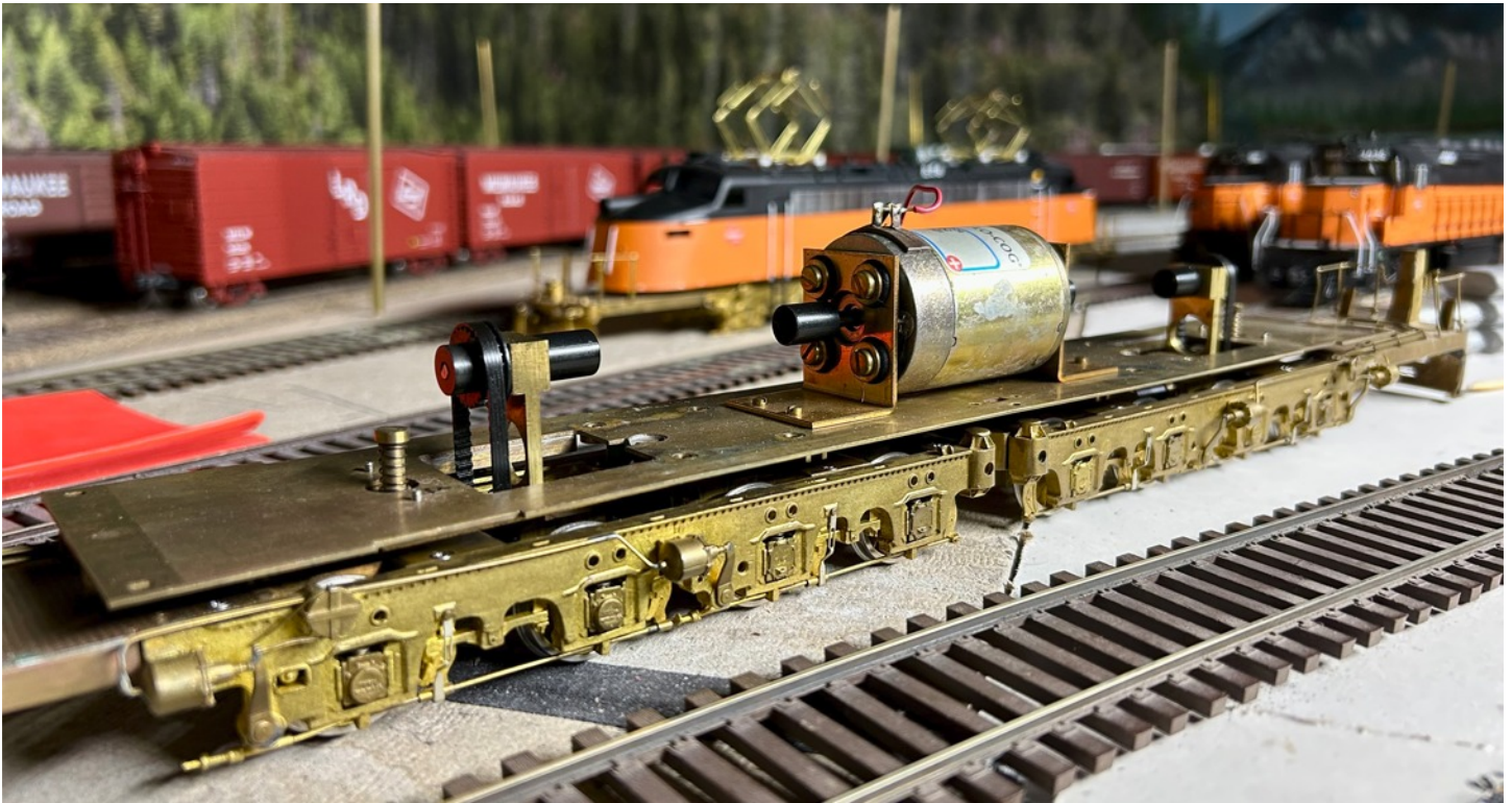
Above: The donor drive ready to install into the newly completed E78 body.
