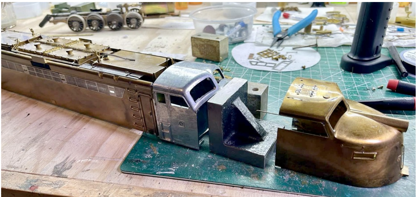
New cab ready for install. Nose will be removed from overland cab
