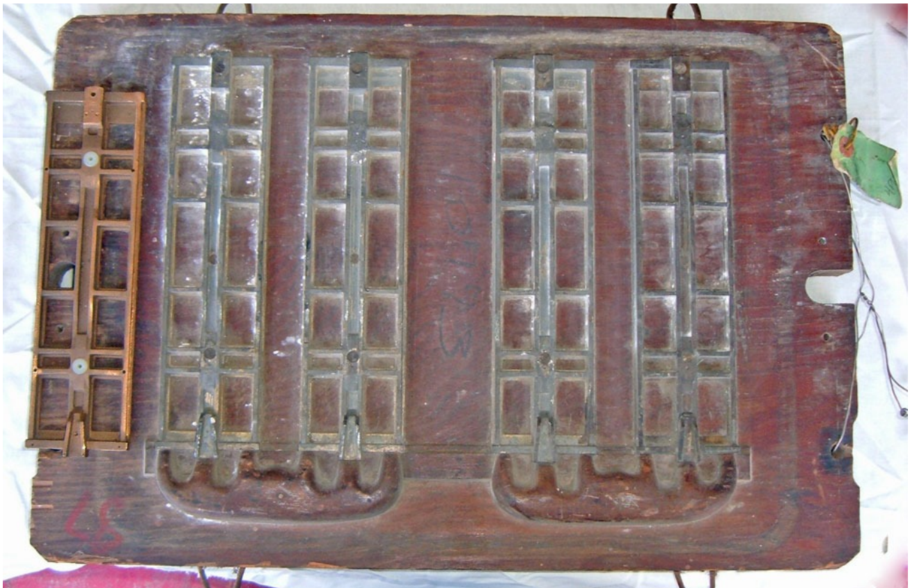
This is another match plate pattern. The frame on the left is from my Lobaugh Berkshire. You can see the similarity. Bob thinks this pattern was for the Lobaugh Challenger tender.
