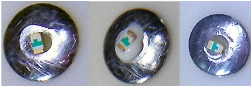
This is MV Products lens after filing with the 603 LED set in place.
