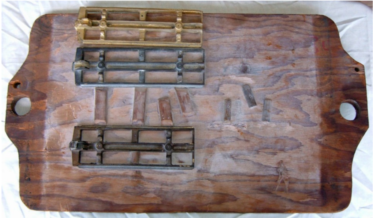
This pattern is an example of a match plate. The parts are one sided and the patterns are mounted on one side of the match plate. The patterns are brass. The gates are wood and you can see them between the parts. This side of the pattern is the cope side. The other side, which is the drag, there is a riser for feeding metal to the gates. At the top is a brass tender frame that came from this pattern. Bob thinks this was a Hines Lines pattern and Henry Pierce probably made it.
