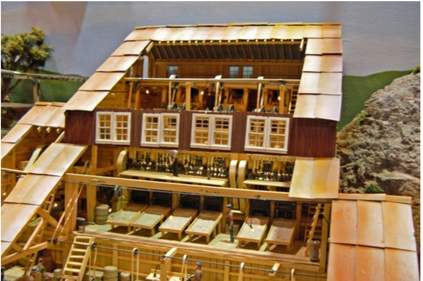
This stamp mill is on section 10, and was built by Dave Connery. Dave left the roof off to show the interior of the mill. The raw ore was loaded in bins at the top. Just below the windows, you can see the stamps for crushing the ore. The crushed ore was then placed on tables just below the stamps for a first sorting. Next the crushed ore was moved to the next level down where it was placed on waffle tables. These tables mimic the prospector panning his ore to separate the gold out. They have an agitation motion that was powered by the line shaft near the bottom of the photo.
