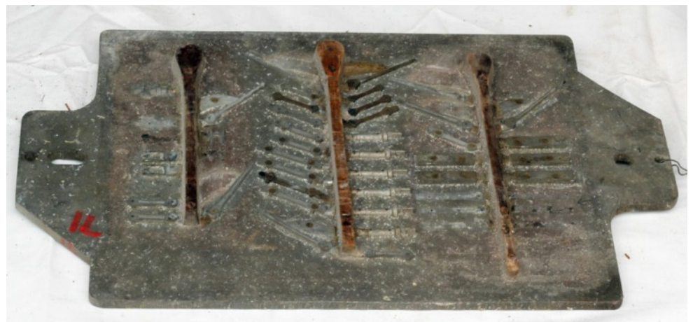
Even the delicate side rods could be sand cast. This pattern is full of them.
