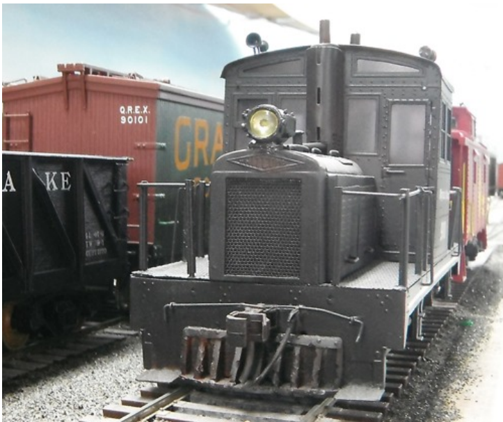
Here is the MV lens installed in the Precision Casting headlight. If you look closely, it almost looks like a bulb in there.
