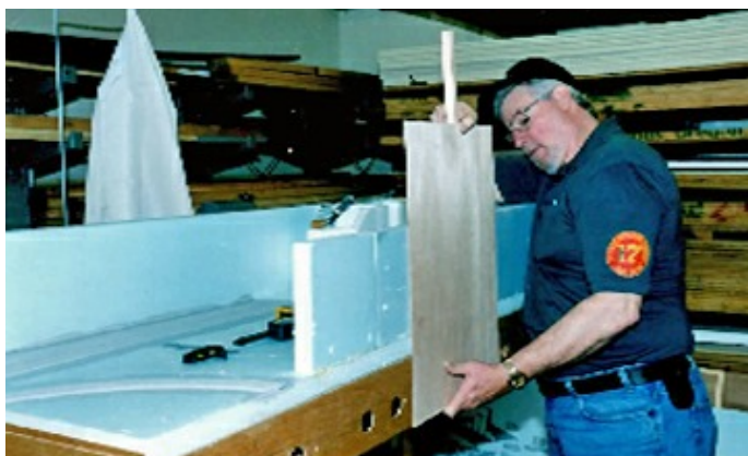
Brad Lloyd applying a door skin. These were used as fascia and helped keep the weight down.
