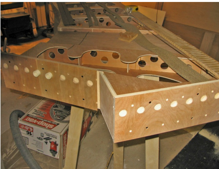
This photo is of another module that Jerry built using the first version of the end plate, pin, and template joining method. Notice that the module construction is a torsion box type of construction with many holes for lightening it. This was to be the start of a branch line and the layout would take off in another direction from here.
