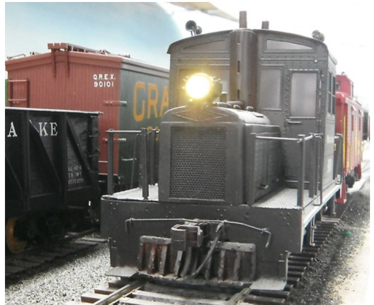
Lights on and by using a warm LED, we get an older incandescent type light.
