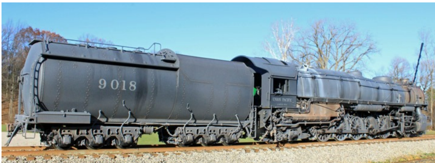
Lee Turner painted this Union Pacific 4-12-2. It looks like the local water has a lot of lime in it as evidenced by the white streaking coming from the pop off valves.
