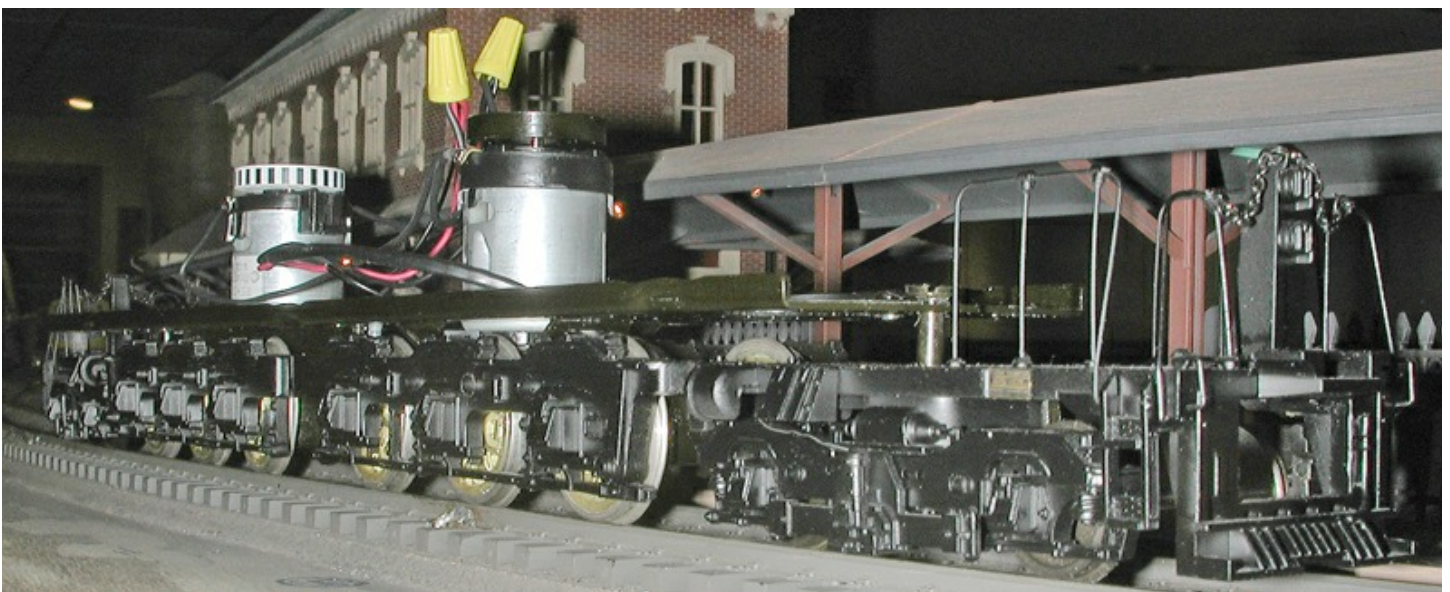
The completed chassis ready for final wiring. It is a good idea to test the locomotive in this state to see if there are any changes that need to be made.
