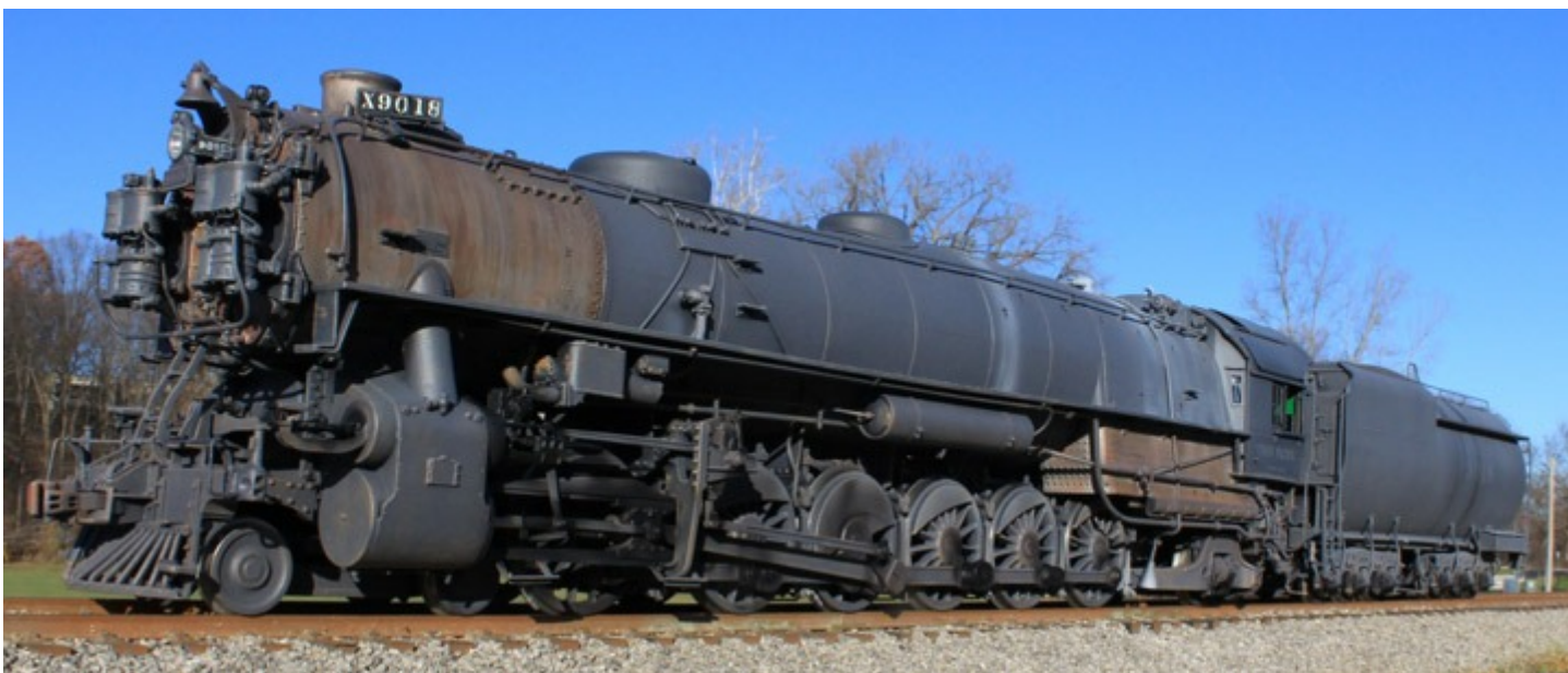
The fireman's side of the Union Pacific 4-12-2. These engines burned a very light low heat coal and needed huge fireboxes to get heat. The coal was so poor that many people said it was like burning dirt. The sides of the track on these lines are full of cinders and ash spewed out by these and other Union Pacific monsters. Lee has captured that in the colors he used around the machinery on this model. The graphite paint used on the fire box and smoke box was not very good and this locomotive is starting to show some uniform rust coming through the paint.
