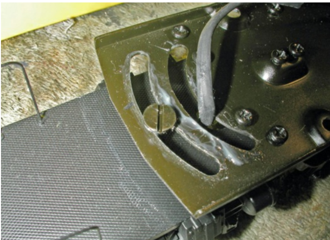
A detail of the chassis showing the front platform flat head slotted pivot screw.
