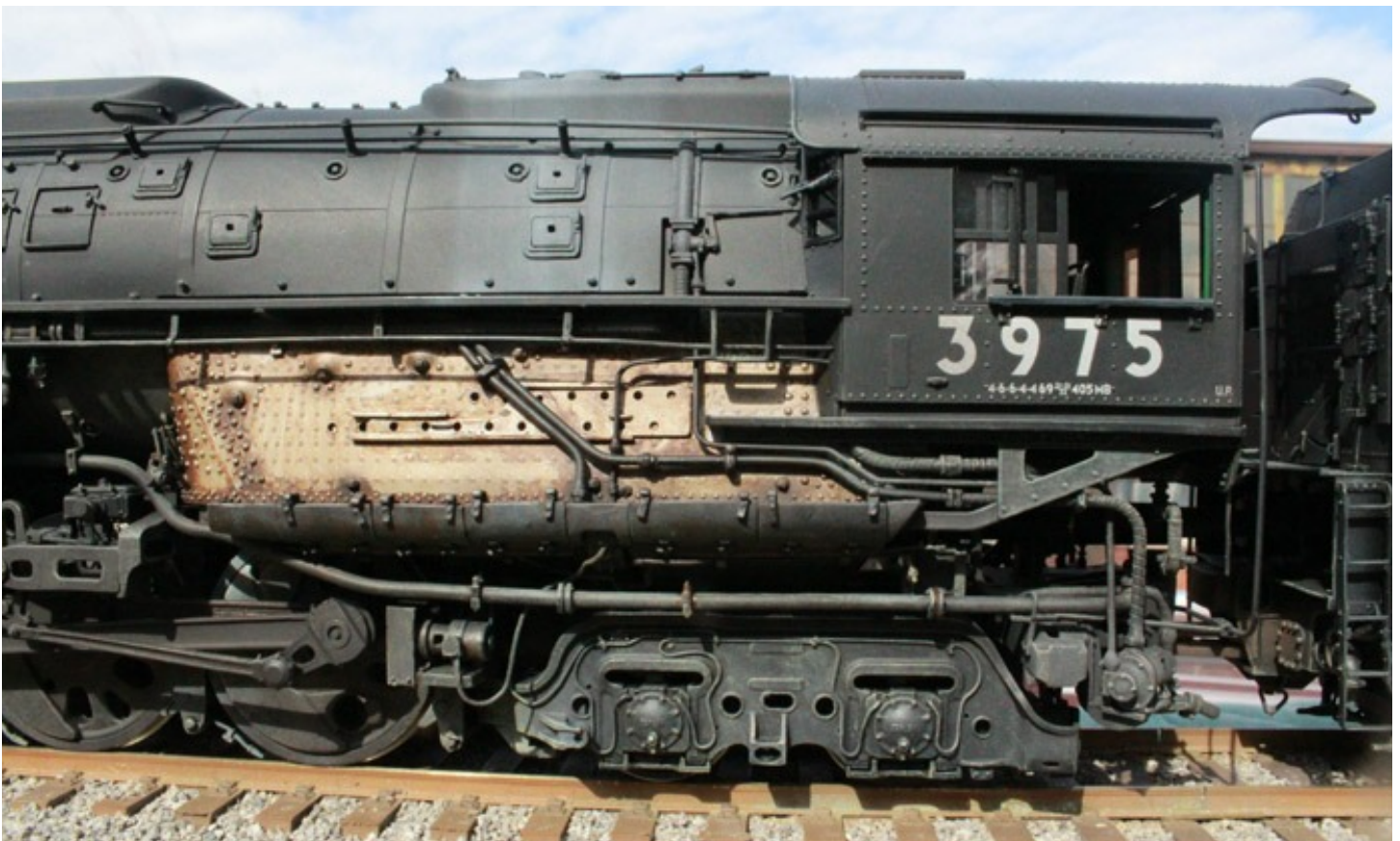
The fireman's side of this Union Pacific Challenger shows how careful and light coats of paint will not cover the detail. This job was done by Lee Turner. There is a lot of work on just the trailing truck, and the washes have brought out a lot of detail.
