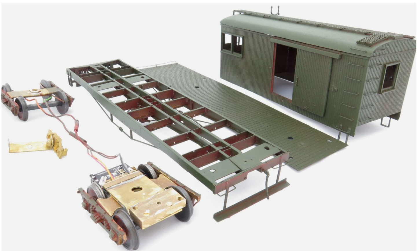
These photos show the model dismantled and after having been spray-painted dark olive green. On the left of the second photo is a typical Kemtron On3 truck set, where the stretcher support needs to be replaced to suit 'O' scale wheels.
