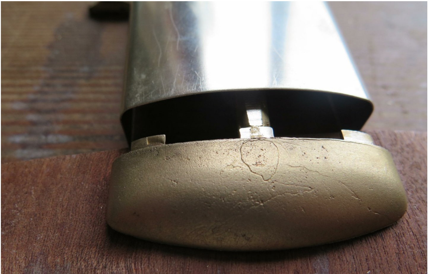
This photo shows the Precision Scale cast roof end for the Mack Rail Bus that Tim used for his model, along with the formed nickel silver roof he made. He next soldered them together and filed the joint and surface smooth.
