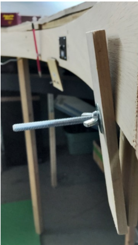
With the laminated fascia being 3/4" and no scrap material at the bottom of the clamp, there is a large V looking opening at the top of the clamp.
