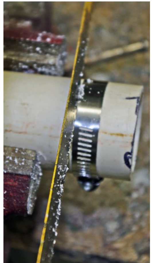
Tank 2 right: I used a hose clamp as a guide for cutting each section the proper length. I used a simple hacksaw. Turn the pipe as you go to assure you are not cutting at an angle.
