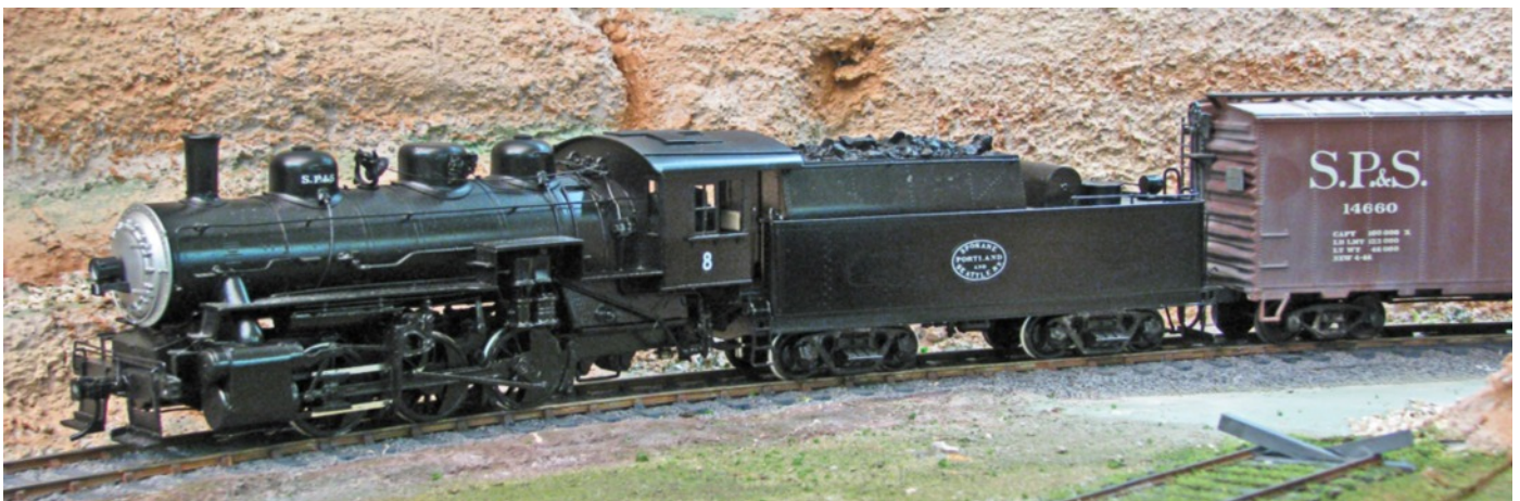
Fresh out of shops, 0-6-0 No.8 is entering Mount Elli yard with a freight. This is a Sunset Models brass U.S.R.A. loco bought 35 years ago that I have painted. The large can motor and toothed belt drive makes it a very powerful and quiet loco. The original Atlas box car behind is one I have painted with extra weight, Athearn trucks and metal wheels.
