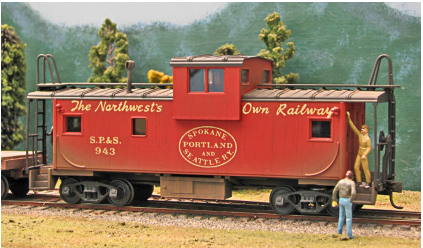
The conductor on caboose No. 943 is receiving instructions from the Station Agent in Mount Elli yard. This is an original Atlas caboose that has been fitted with extra weight, metal trucks and wheels, then painted to represent one of the SP&S more modern cabooses.
