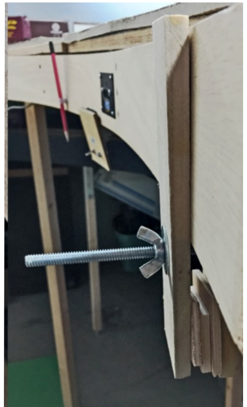
If you need a wider area, such as this fascia, simply flip the clamp upside down with the shorter portion of the clamp at the bottom.
