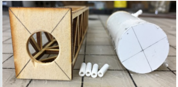
Figure 8 above and 9 below show the hole cut into the tank base, along with small pieces of styrene tubing used for the legs or standoffs.
