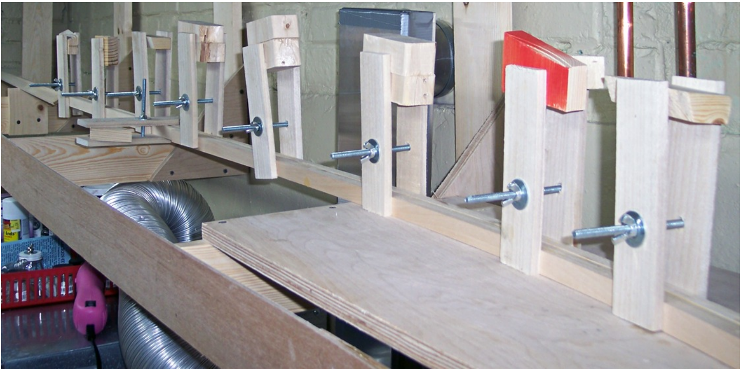
This shows the clamped spline while gluing. Notice here that I used the shorter end for the clamp and large scrap stock for the other end. This provided me with more strength on the clamping end.
