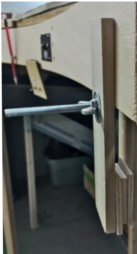
By adding some scrap wood at the bottom of the clamp, roughly equal to the material being clamped, there is now a full flat clamping surface
