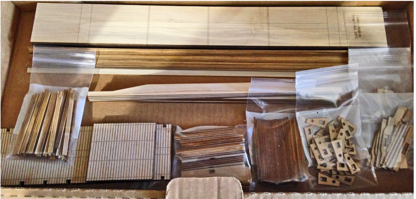
Using that wood and some birch plywood, I found a plan on the Internet and designed all the parts in my computer. Using my laser cutter, I cut and engraved all the parts.
