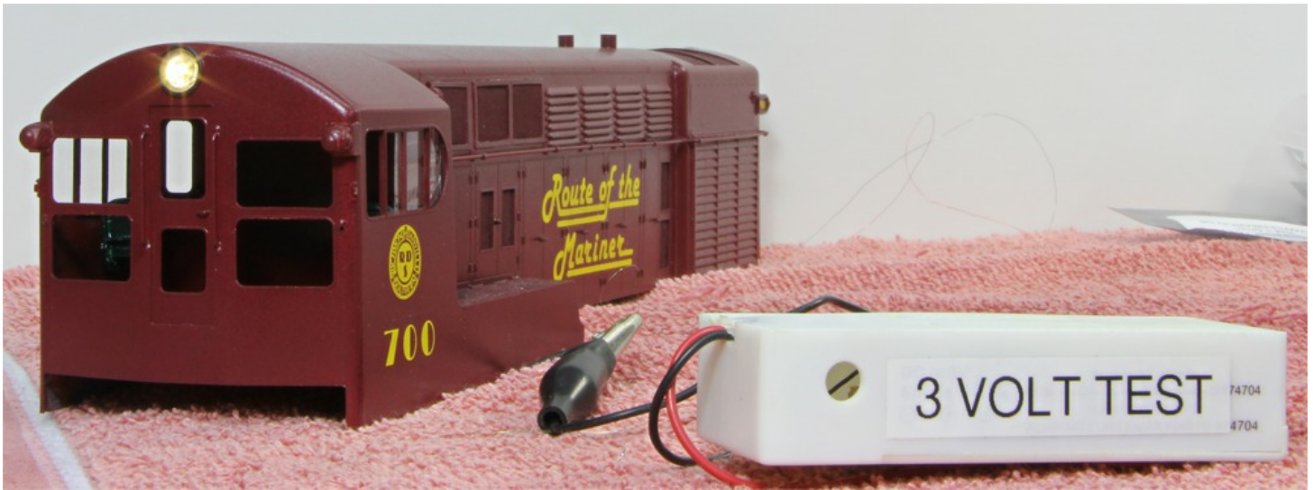
One last test to be sure the connectors are soldered properly and all lights work.
