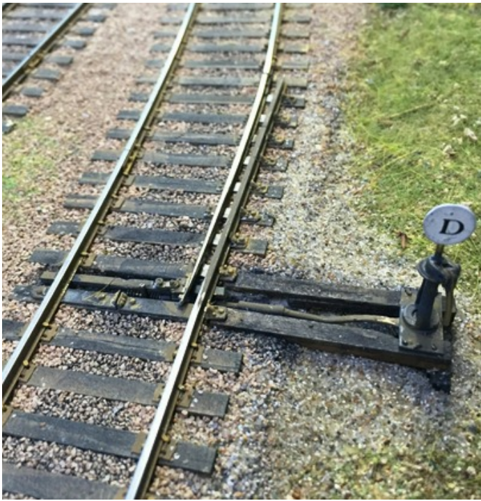
Operating split rail derail, code 125. Code 100 also available in either right hand or left.
