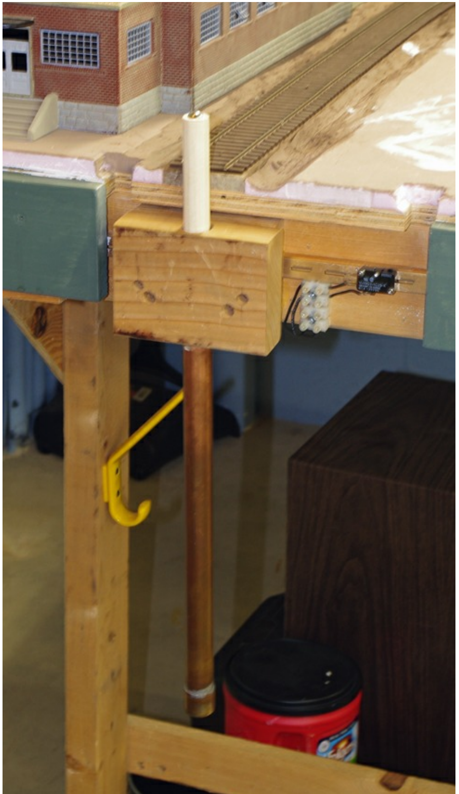
I liked this idea. The wood block is the rest for the lift out section. There is a copper water pipe in it with a cap on it. Inside the copper pipe is a door spring. Then, a wood dowel gets dropped into the copper pipe. When the bridge is lowered, it forces the dowel into the copper pipe. When the bridge is raised, the spring forces the wood dowel up and the track is protected. No more forgetting to protect the track and driving the train to the floor. The lift bridge at Jorgenson is protected the same way.
