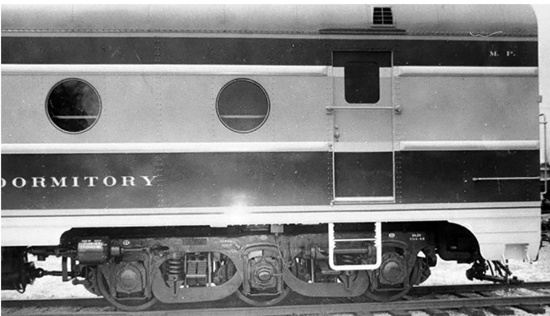
Six wheel trucks with in board mounted brake cylinder. These were very unique trucks similar to some used on the NYC 20th Century cars.
