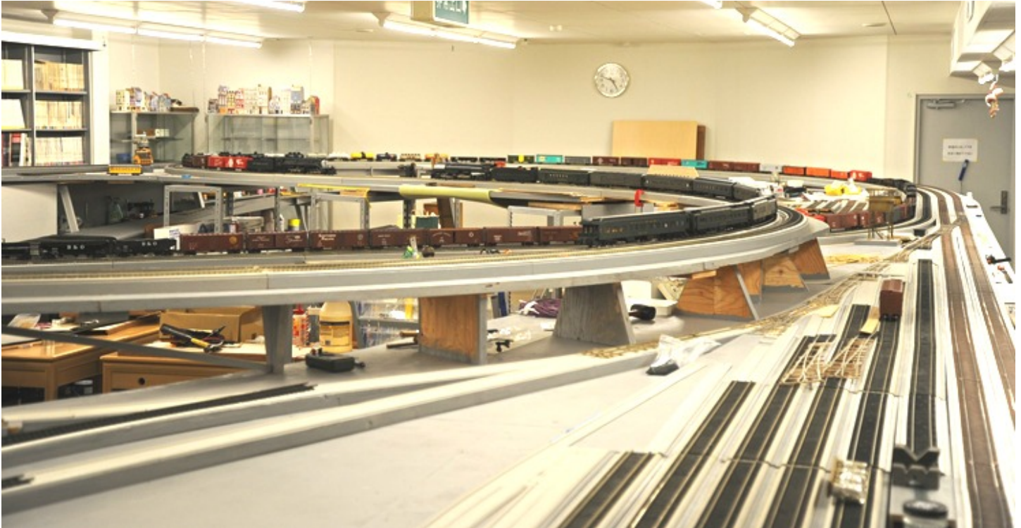
Shot of the museum under construction. Pictured is a 100 car freight train with all cars equipped with Tad's very low friction wheel contour pulled by a single steam engine. This engine can pull 117 cars on this layout at less than 1 Amp draw. 90% of the cars are brass – old Max Gray, US Hobby and custom-built by Tad. This layout has 1.56% grade.
