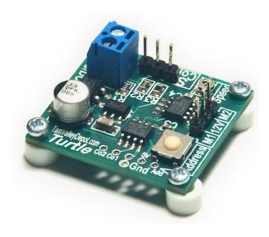
It has a built in DCC accessory decoder that "learns" addresses at the push of the Address button. No programming CVs. A second address is used as a Local Lock Out function so you can disable the Fascia Controller for use on CTC layouts where the dispatcher must release certain turnouts. See their Website for more details.
