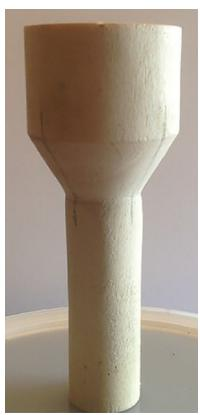
Mold for pots turned on lathe.
