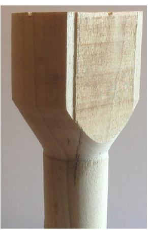
Divider flat cut, with rivet flange relief.
