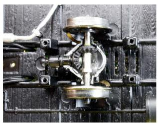
On30 Bachmann RAIL TRUCK replacement gears #2805-6. Fits the Bachmann On30 RAIL TRUCK - Set of three steel lineshaft gears to replace the factory plastic lineshaft gears, which are prone to breakage. The kit includes 6 gears and step-by-step instructions for installation.
