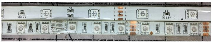
Top shows 30 LEDs per meter vs 60 LEDs on bottom.
