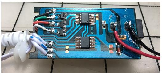
Inside the controller box. I used a new red and black wire for the 12 volts. The white, red, green, black wires on the upper left were cut and spliced with the furnace wire making note of the color swap and must importantly making sure which of the four is +12 In my case it was always the white wire.
