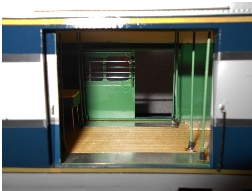
Figure 18 left: Working baggage door with steel window bars, wood flooring finished with clear poly coat and vertical safety bars.
