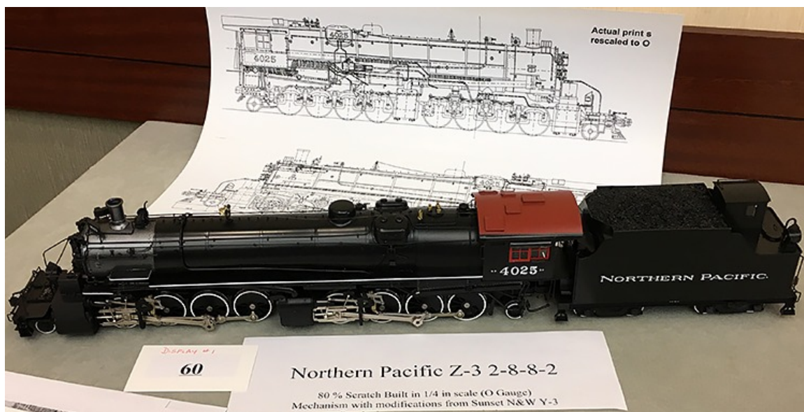
Dale DeWitt's Northern Pacific Z-3 2-8-8-2 was 80% scratch built. Mechanism with modifications from a Sunset N&W Y-3.
