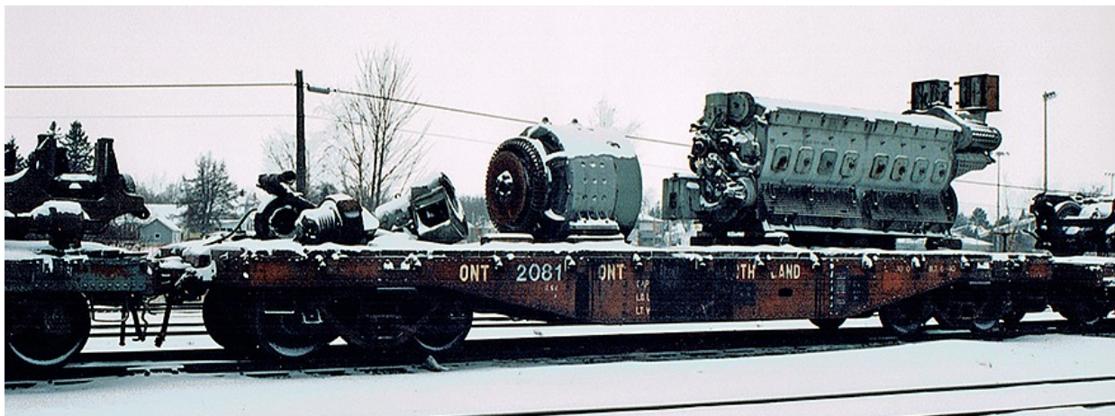
Parts and pieces of GP9 No. 1601 loaded on flat cars in North Bay, ONT. on December 29, 1993. This unit has since been rebuilt, and is back in service.
