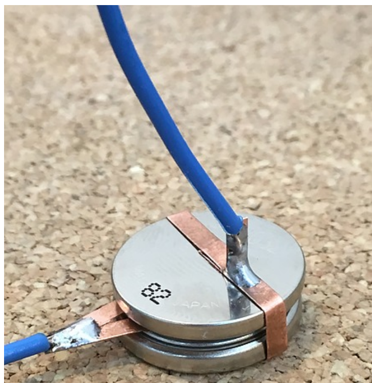
Because battery holders take up a lot of room, I fabricated feeders using copper strips. To secure them, I used two-part epoxy resin. If space is not a concern, wired holders are readily available.
