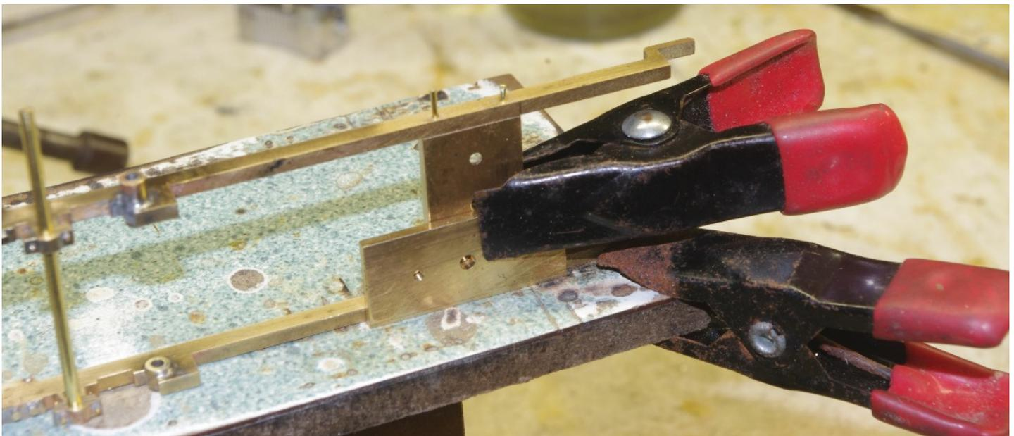
*This is how I soldered the front of the frame under the cylinders together. Notice the pins again. I will file them off next.*
