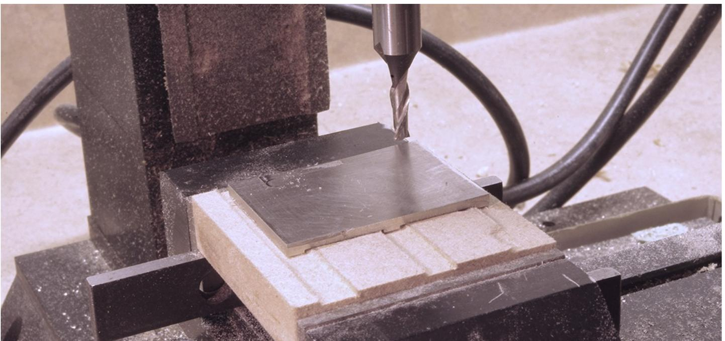
*In this operation, I am doing the other side of my part. Notice how I cut the wood to fit the profile of the first piece. After cutting the wood, do not remove it from the vise since the cuts in the wood are now registration lines for gluing the nickel silver back to the wood. These features I am cutting are largely for looks and this registration works just fine.*
