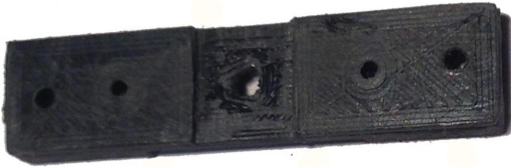
The new bolster. The square for the distance piece has been narrowed to 8mm.
