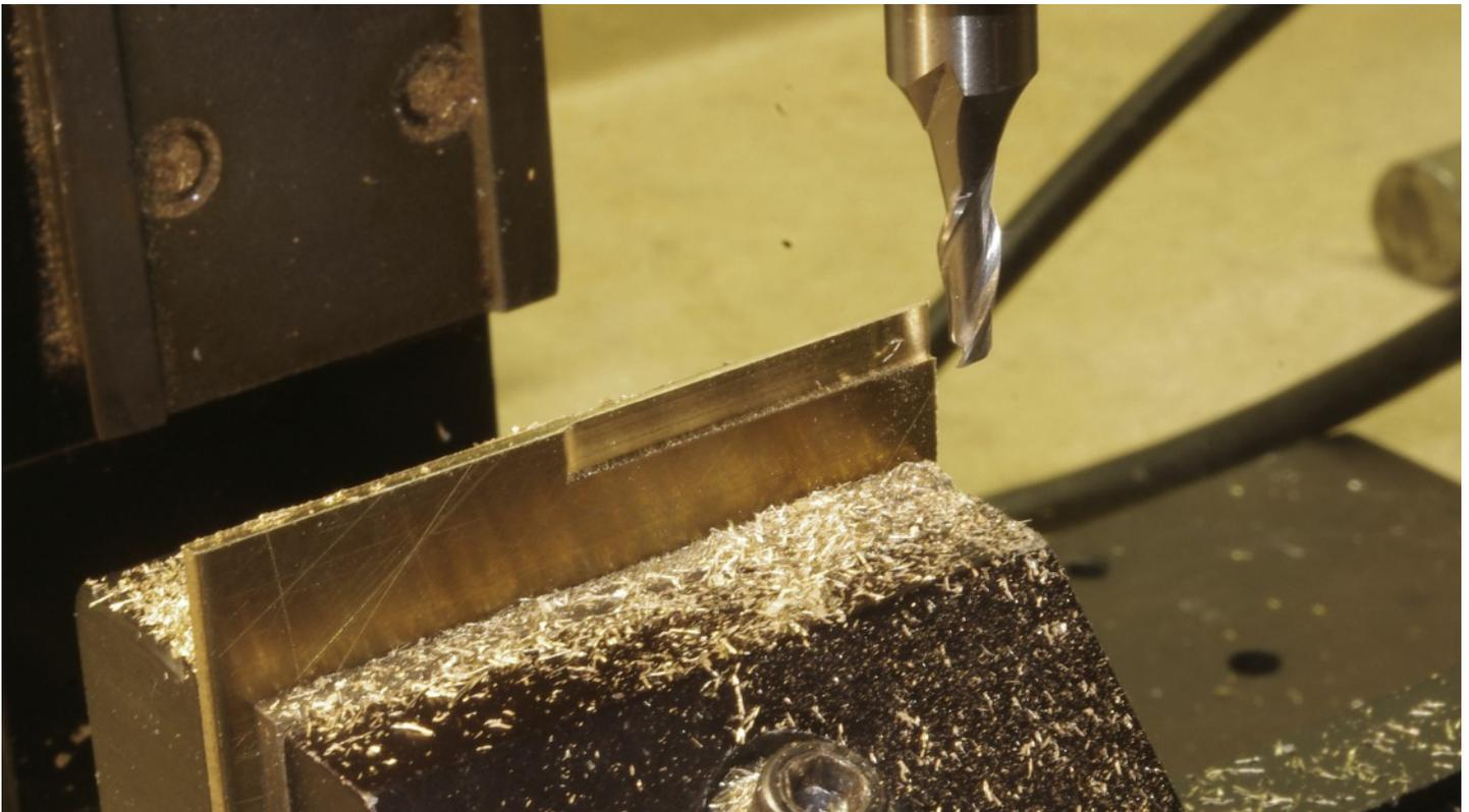
*Part of the spring rigging had a small “T” shaped piece. I put a piece of brass plate in the vise as shown and cut on each side of it as shown. After this, I cut off a piece of this for the next operation which is in the next photo. You will get the idea when you look at that photo.*
